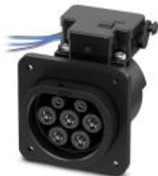
Infrastructure Socket Outlet for charging electric vehicles with alternating current (AC), compatible with Infrastructure Plugs, GB/T, GB/T 20234.2-2015, 32 A / 440 V (AC), 12 V Locking actuator, Single wires, length: 0.7 m, Rear panel mounting
