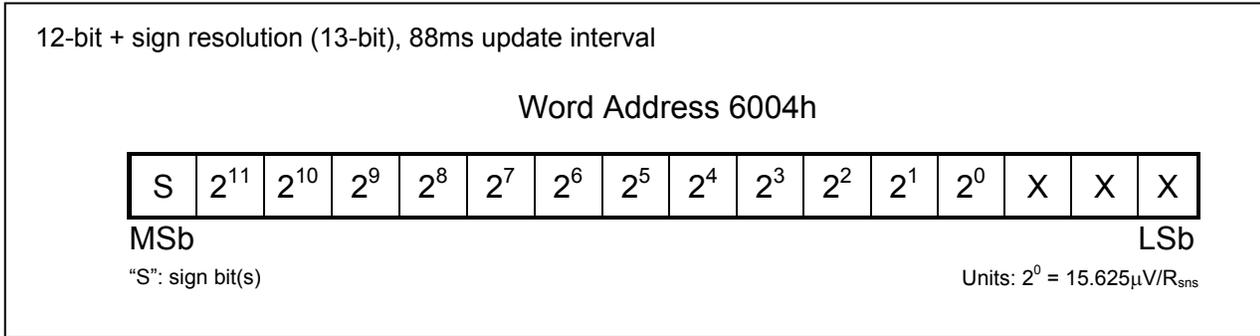
**Figure 12. Average Current Register Format**
