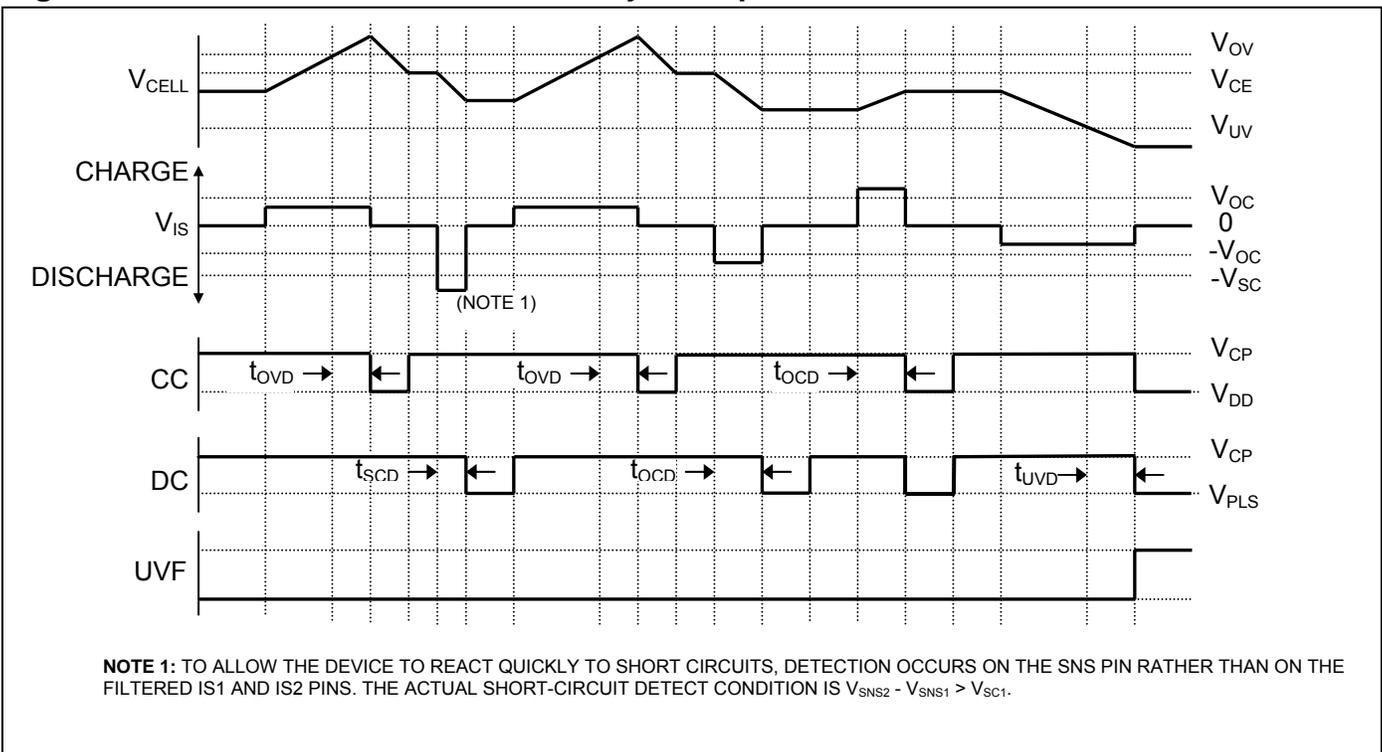
**Summary.** All of the protection conditions described above are AND'ed together with temperature protection functions to affect the CC and DC outputs.
