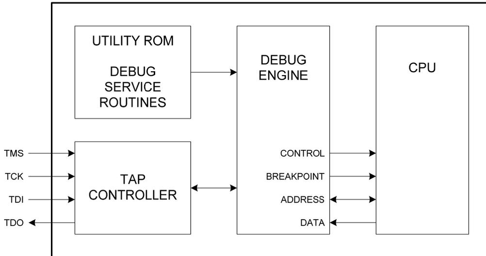
The embedded hardware debug engine is an independent hardware block in the microcontroller. The debug engine can monitor internal activities and interact with selected internal registers while the CPU is executing user code. Collectively, the hardware and software features allow two basic modes of in-circuit debugging:
