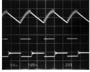
20µs/DIV 1704 G07 CH1: V<sub>OUTSW</sub> = 1.8V, AC 20mV/DIV CH2: V<sub>TG</sub>, 5V DIV
