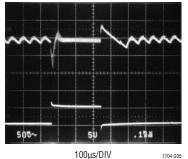
100µs/DIV CH1: V<sub>OUTSW</sub> = 1.8V, AC 50mV/DIV CH2: 0.5A to 5.5A LOAD, 5A DIV
