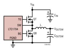
Figure 1. Synchronous Buck Architecture
