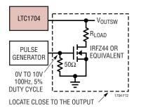
Figure 12. Transient Load Generator
