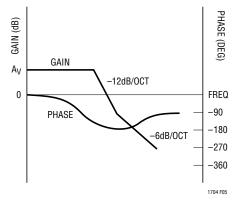
Figure 7. Transfer Function of Buck Modulator
