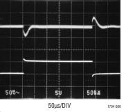
CH1: V<sub>OUTSW</sub> = 1.8V, AC 50mV/DIV CH2: 5A to 10A LOAD, 5A DIV
