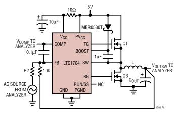
Figure 11. Modulator Gain/Phase Measurement Setup
