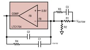
Figure 3. "Type 3" Feedback Loop
