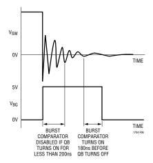
Figure 6. Burst Comparator Turns On 180ns Before QB Turns Off 1704bfa
