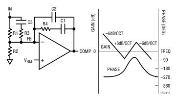
Figure 10. Type 3 Schematic and Transfer Function
