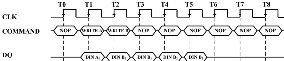
**Figure 11. Write Interrupted by a Write (Burst Length = 4)**
