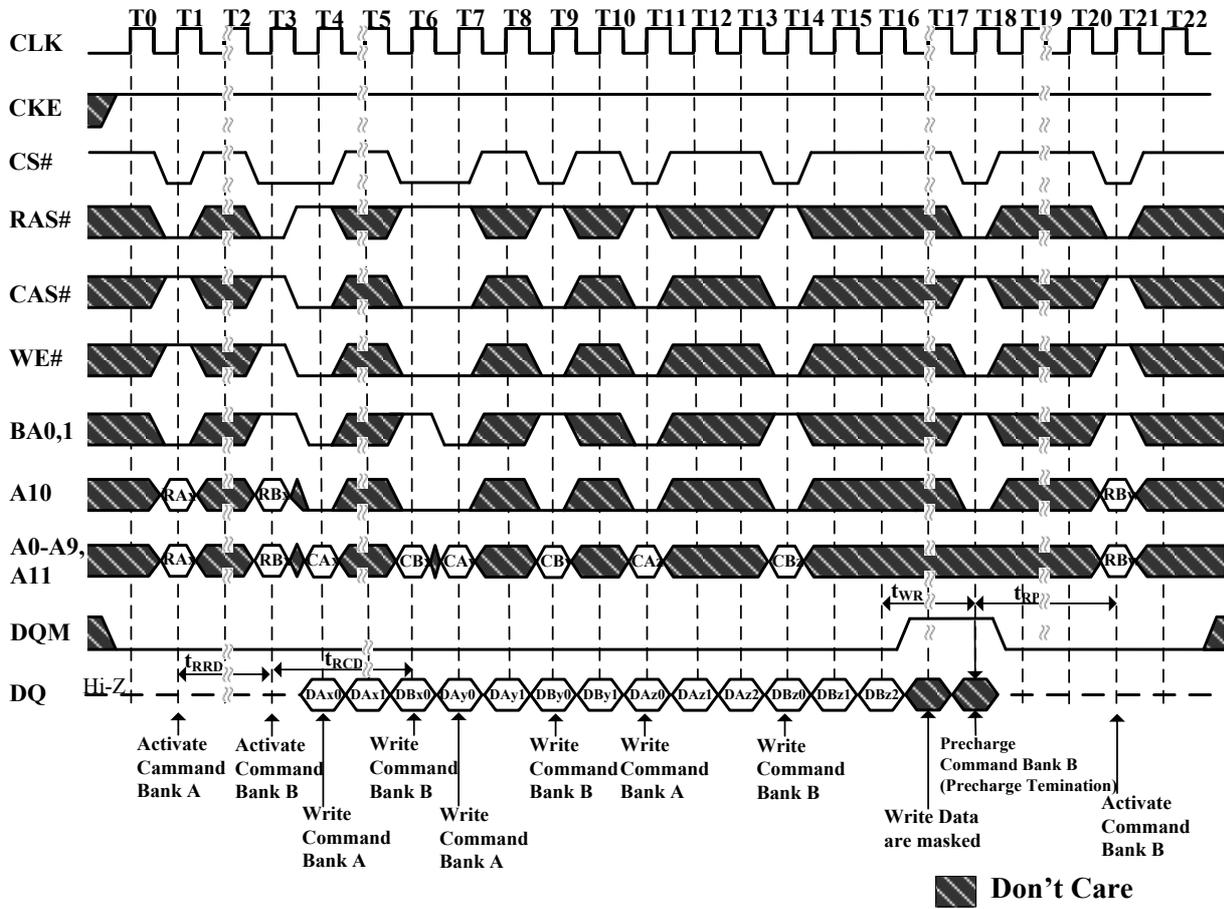
**Figure 42. Precharge Termination of a Burst**
