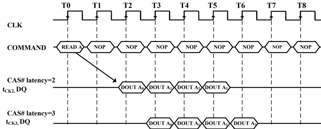
**Figure 4. Burst Read Operation (Burst Length = 4, CAS# Latency = 2, 3)**
