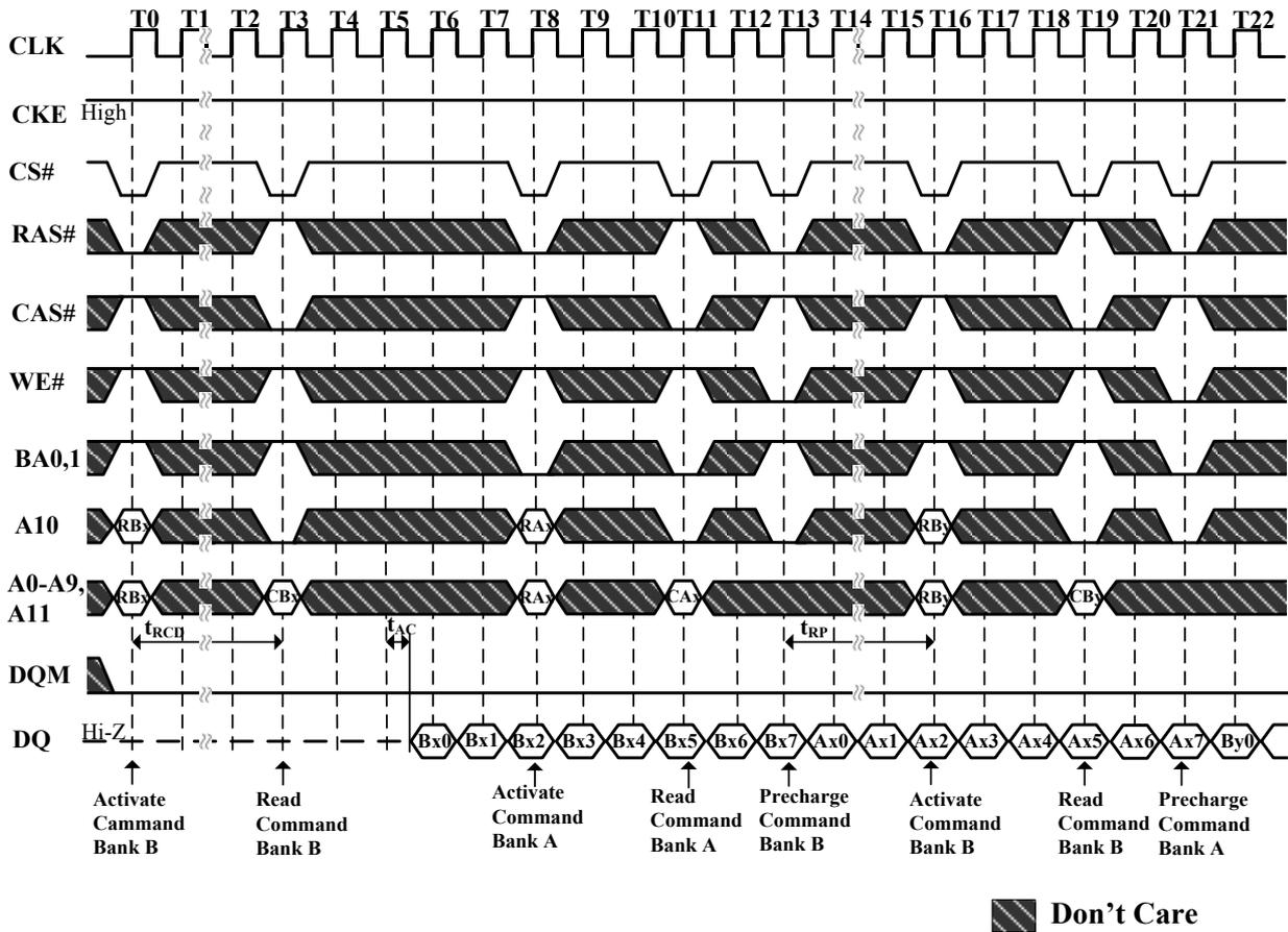
**Figure 30. Random Row Write (Interleaving Banks)**
