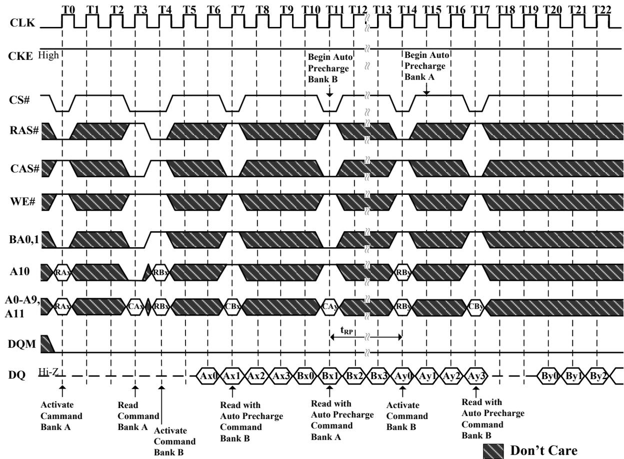
**Figure 35. Auto Precharge after Write Burst (Burst Length=4)**
