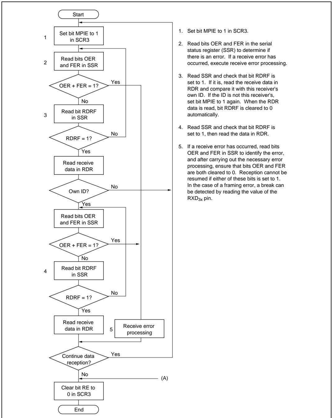
Figure 10.19 Example of Multiprocessor Data Reception Flowchart
