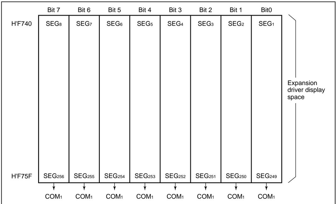
**Figure 13.12 LCD RAM Map when Using Segment External Expansion
