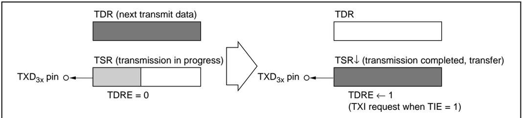
**Figure 10.2 (b) TDRE Setting and TXI Interrupt**
