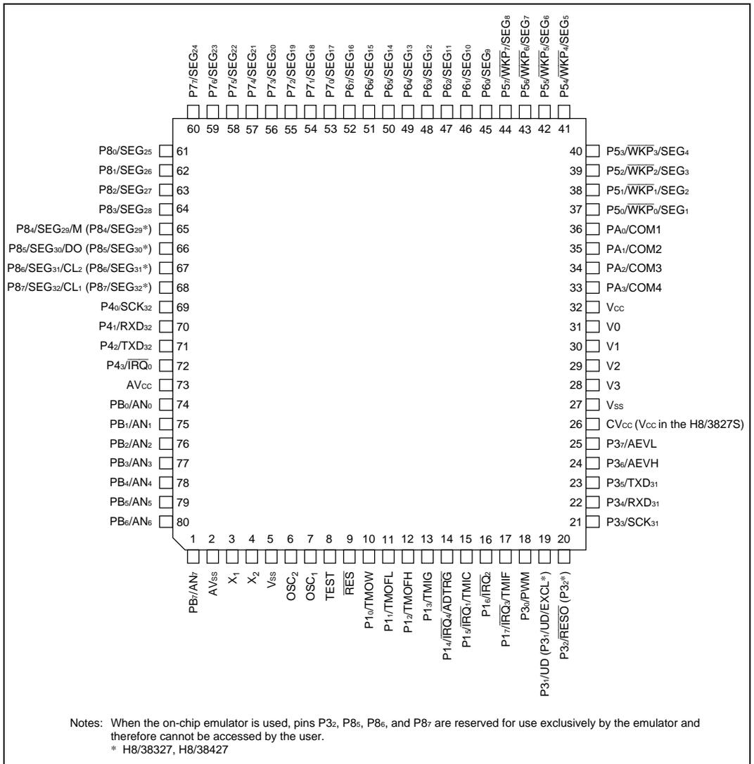
**Figure 1.2 Pin Arrangement (FP-80A, TFP-80C: Top View)**
