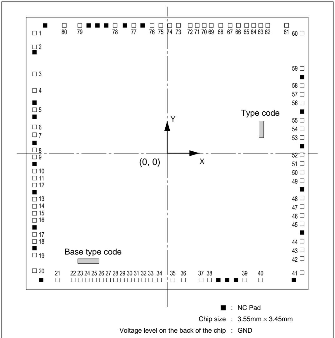
**Figure 1.5 Bonding Pad Location Diagram of H8/3827S Group (Mask ROM Version)
