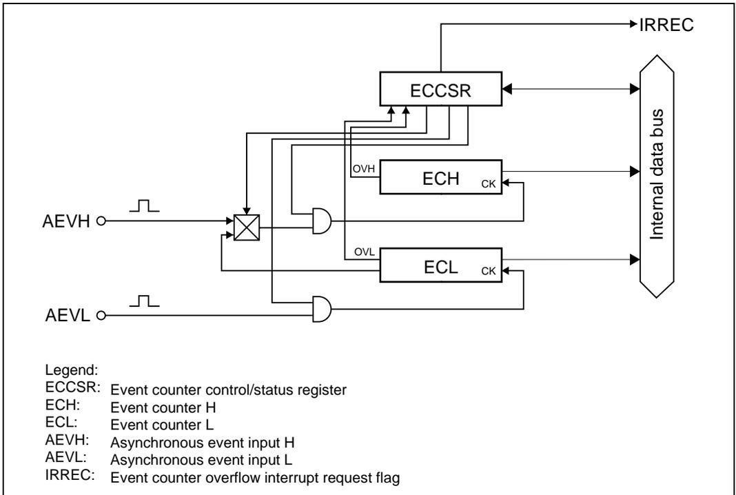
**Figure 9.19 Block Diagram of Asynchronous Event Counter**
