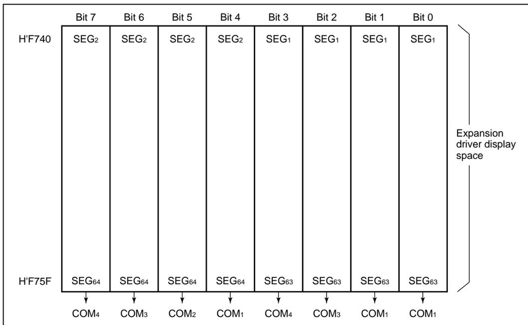
**Figure 13.9 LCD RAM Map when Using Segment External Expansion
