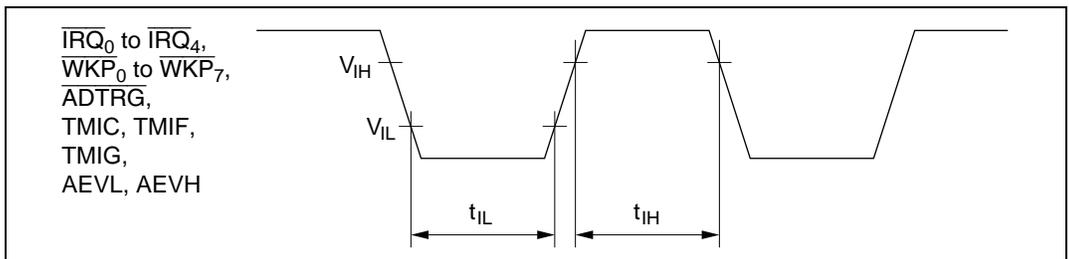
**Figure 15.3 Input Timing**
