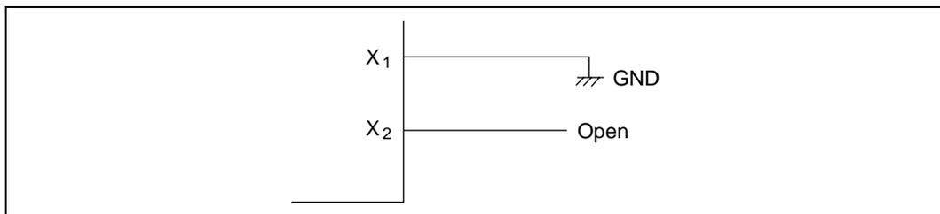
**Figure 4.8 Pin Connection when not Using Subclock**
