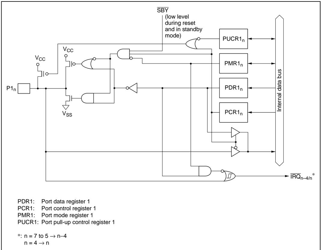
Figure C.1 (a) Port 1 Block Diagram (Pins P1<sub>7</sub> to P1<sub>4</sub>)
