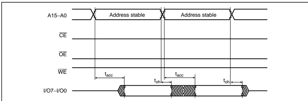
**Figure 6.15  $\overline{\text{CE}}$  and  $\overline{\text{OE}}$  Enable State Read Timing Waveforms**
