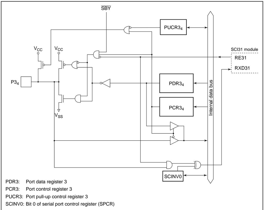
**Figure C.2 (c) Port 3 Block Diagram (Pin P3<sub>4</sub>)**
