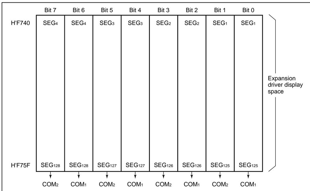
**Figure 13.11 LCD RAM Map when Using Segment External Expansion
