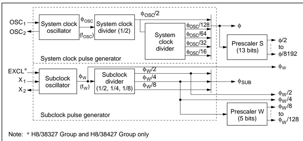
**Figure 4.1 Block Diagram of Clock Pulse Generators**
