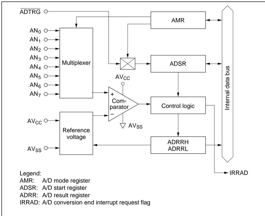
**Figure 12.1 Block Diagram of the A/D Converter**
