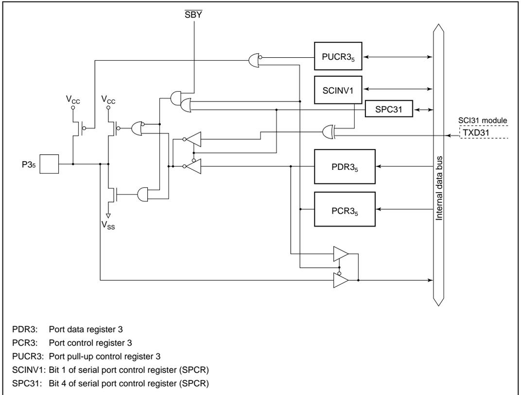
**Figure C.2 (b) Port 3 Block Diagram (Pin P3<sub>5</sub>)**
