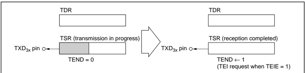
**Figure 10.2 (c) TEND Setting and TEI Interrupt**
