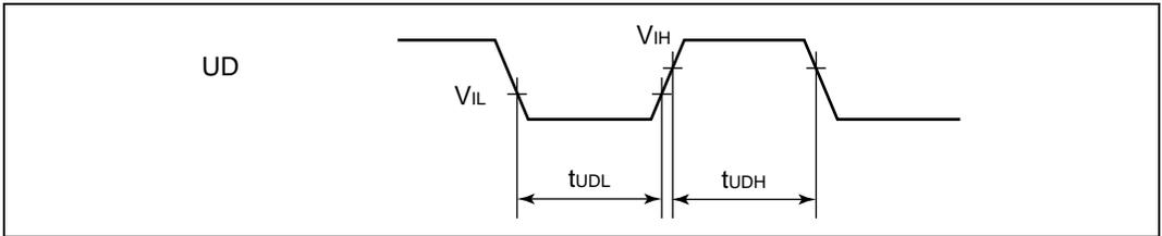
**Figure 15.4 UD Pin Minimum Modulation Width Timing**
