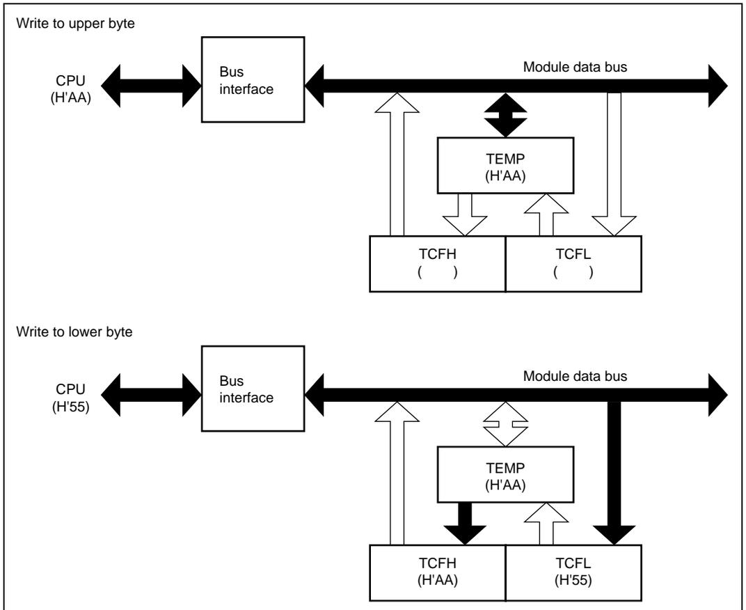
**Figure 9.4 Write Access to TCR (CPU → TCF)**
