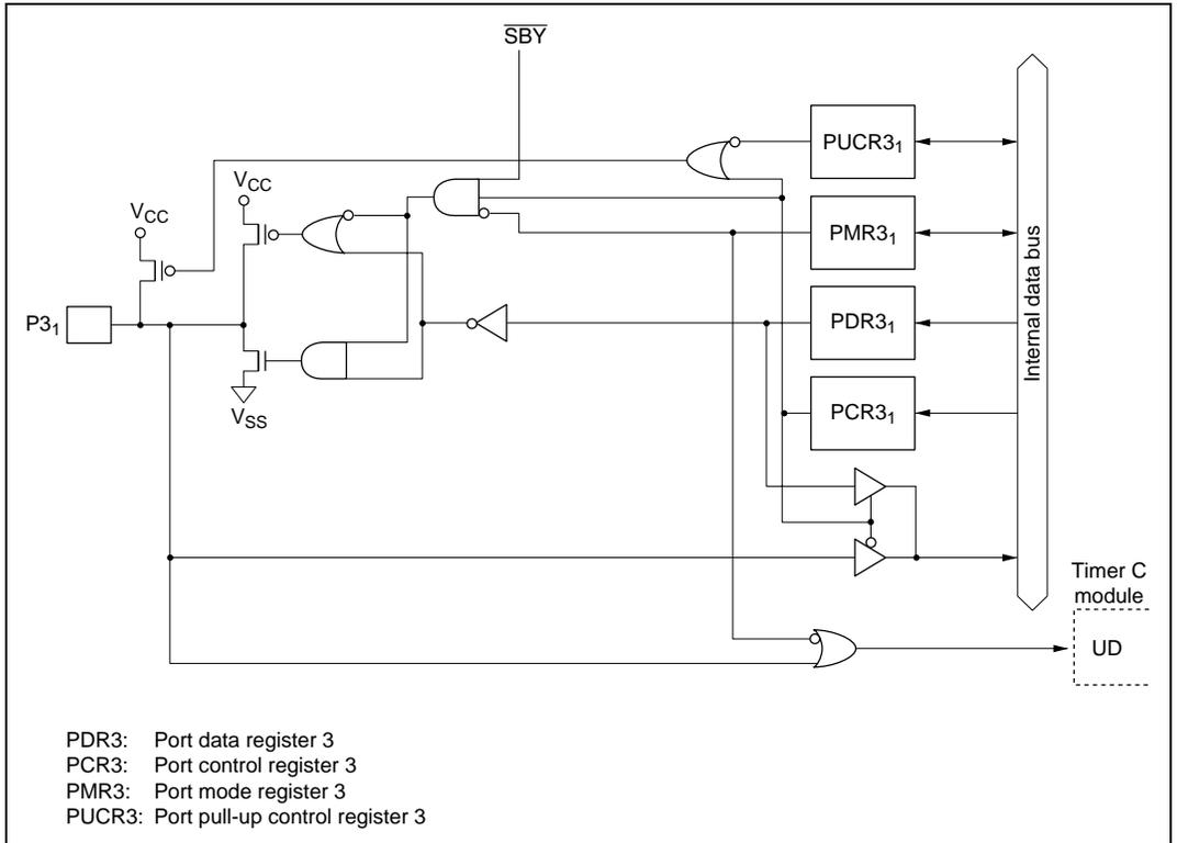
**Figure C.2 (f-1) Port 3 Block Diagram (Pin P3<sub>1</sub>, H8/3827R Group and H8/3827S Group)**
