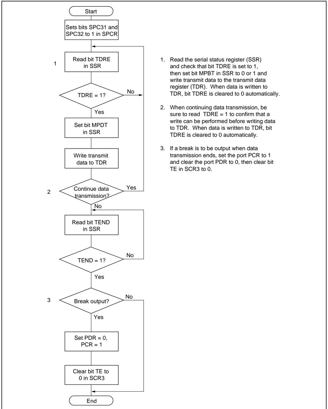
Figure 10.17 Example of Multiprocessor Data Transmission Flowchart
