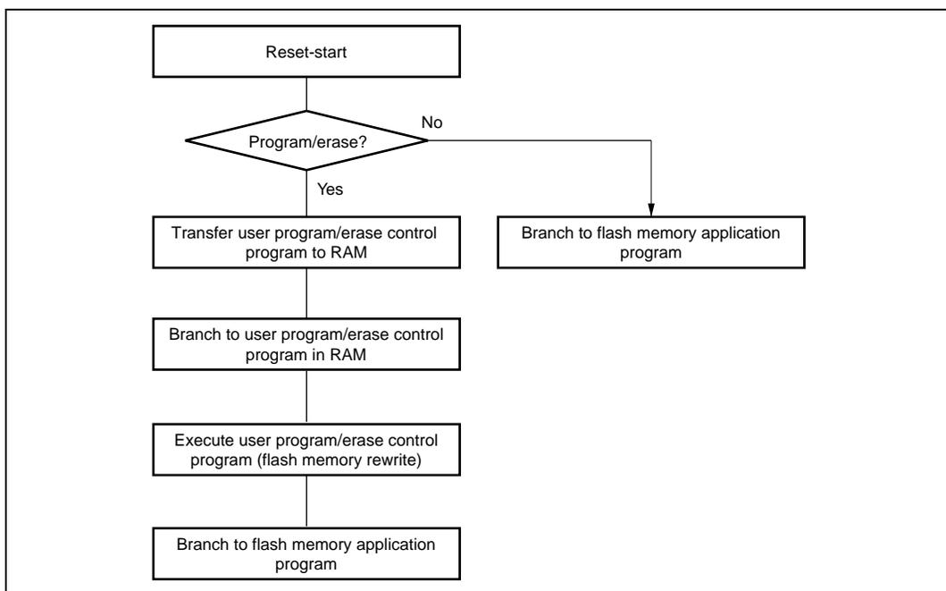
**Figure 6.9 Programming/Erasing Flowchart Example in User Program Mode**
