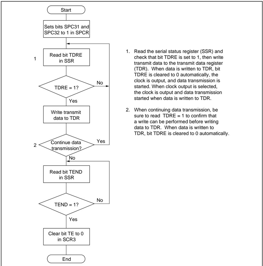
**Figure 10.11 Example of Data Transmission Flowchart (Synchronous Mode)**
