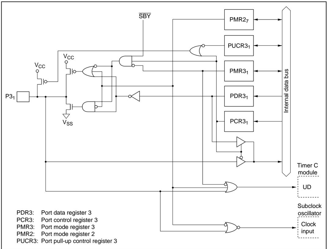
**Figure C.2 (f-2) Port 3 Block Diagram (Pin P3<sub>1</sub>, H8/38327 Group and H8/38427 Group)**
