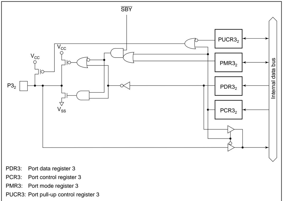
**Figure C.2 (e-2) Port 3 Block Diagram (Pin P3<sub>2</sub> in the Mask ROM Version of the H8/38327 Group and H8/38427 Group)**
