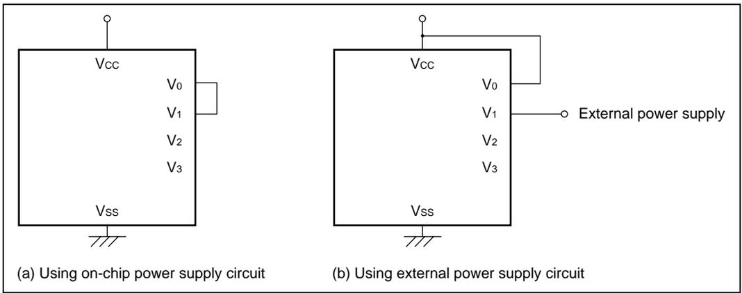
**Figure 13.4 Examples of LCD Power Supply Pin Connections**
