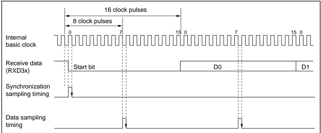
**Figure 10.21 Receive Data Sampling Timing in Asynchronous Mode**
