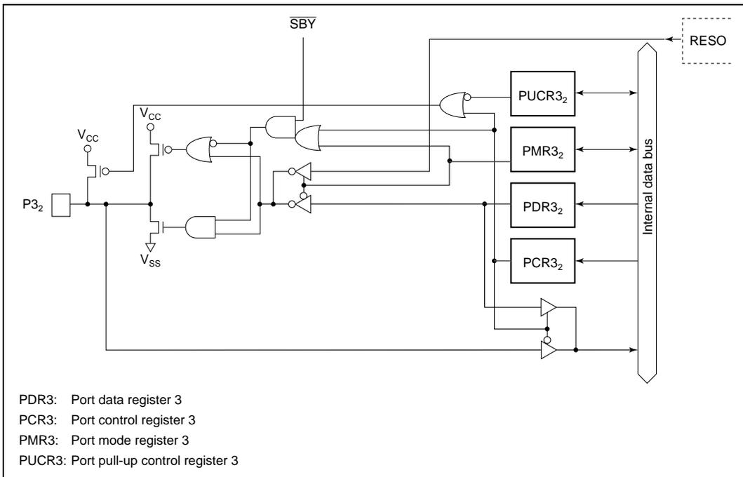
**Figure C.2 (e-1) Port 3 Block Diagram (Pin P3<sub>2</sub>, H8/3827R Group and H8/3827S Group)**
