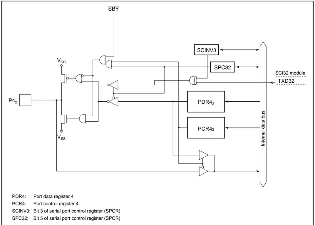
**Figure C.3 (b) Port 4 Block Diagram (Pin P4<sub>2</sub>)**
