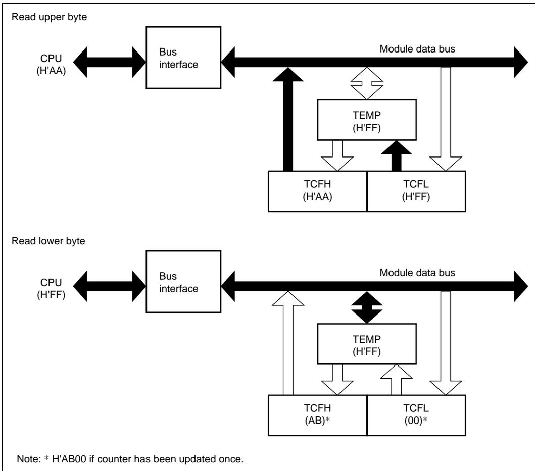
**Figure 9.5 Read Access to TCF (TCF → CPU)**
