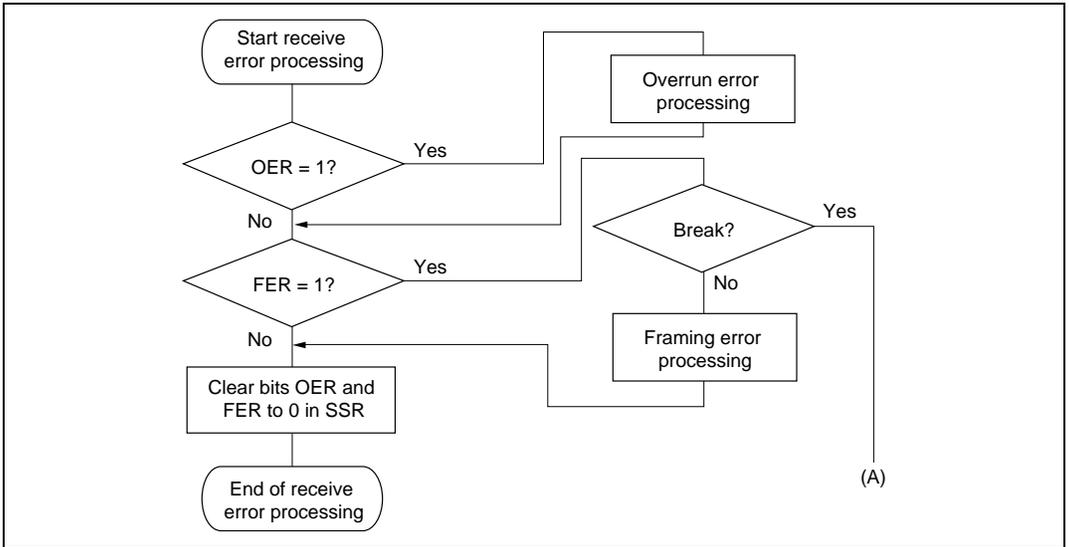
**Figure 10.19 Example of Multiprocessor Data Reception Flowchart (cont)**
