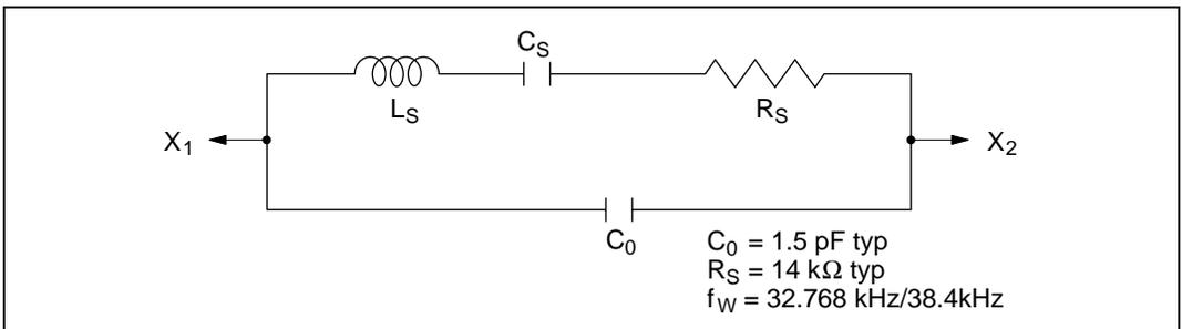
**Figure 4.7 Equivalent Circuit of 32.768 kHz/38.4 kHz Crystal Oscillator**
