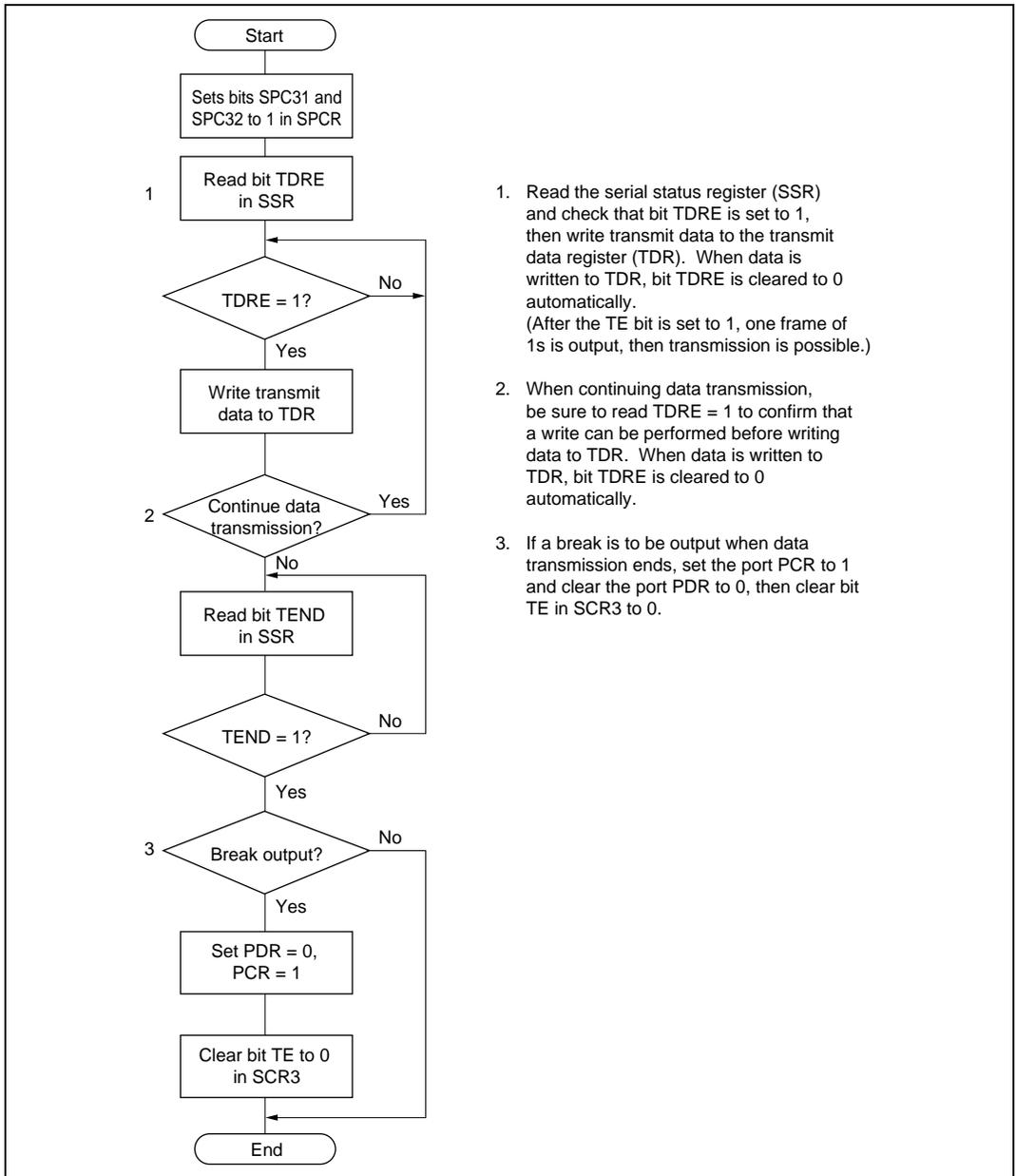
**Figure 10.6 Example of Data Transmission Flowchart (Asynchronous Mode)**
