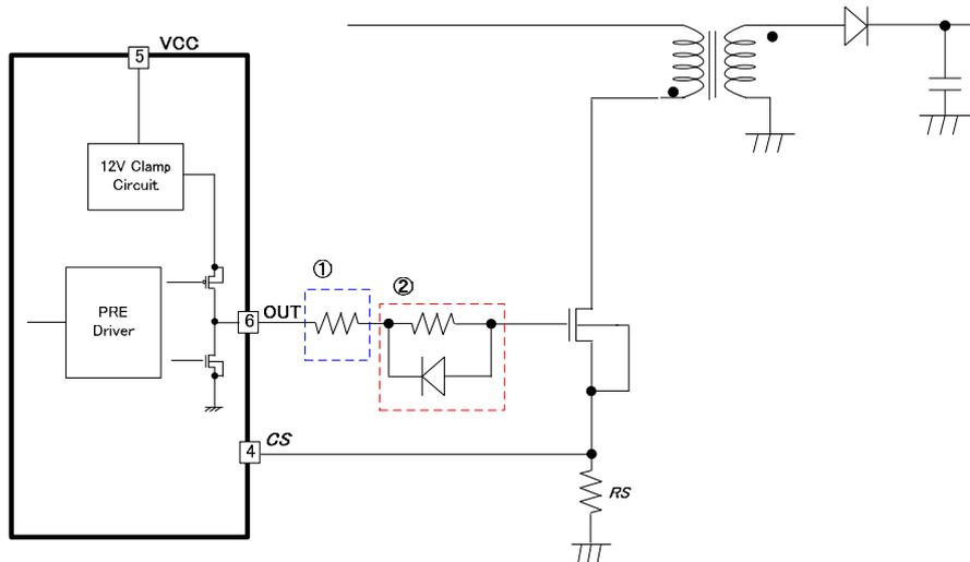
Figure 26. OUT Pin (Pin 5) Driver Circuit
