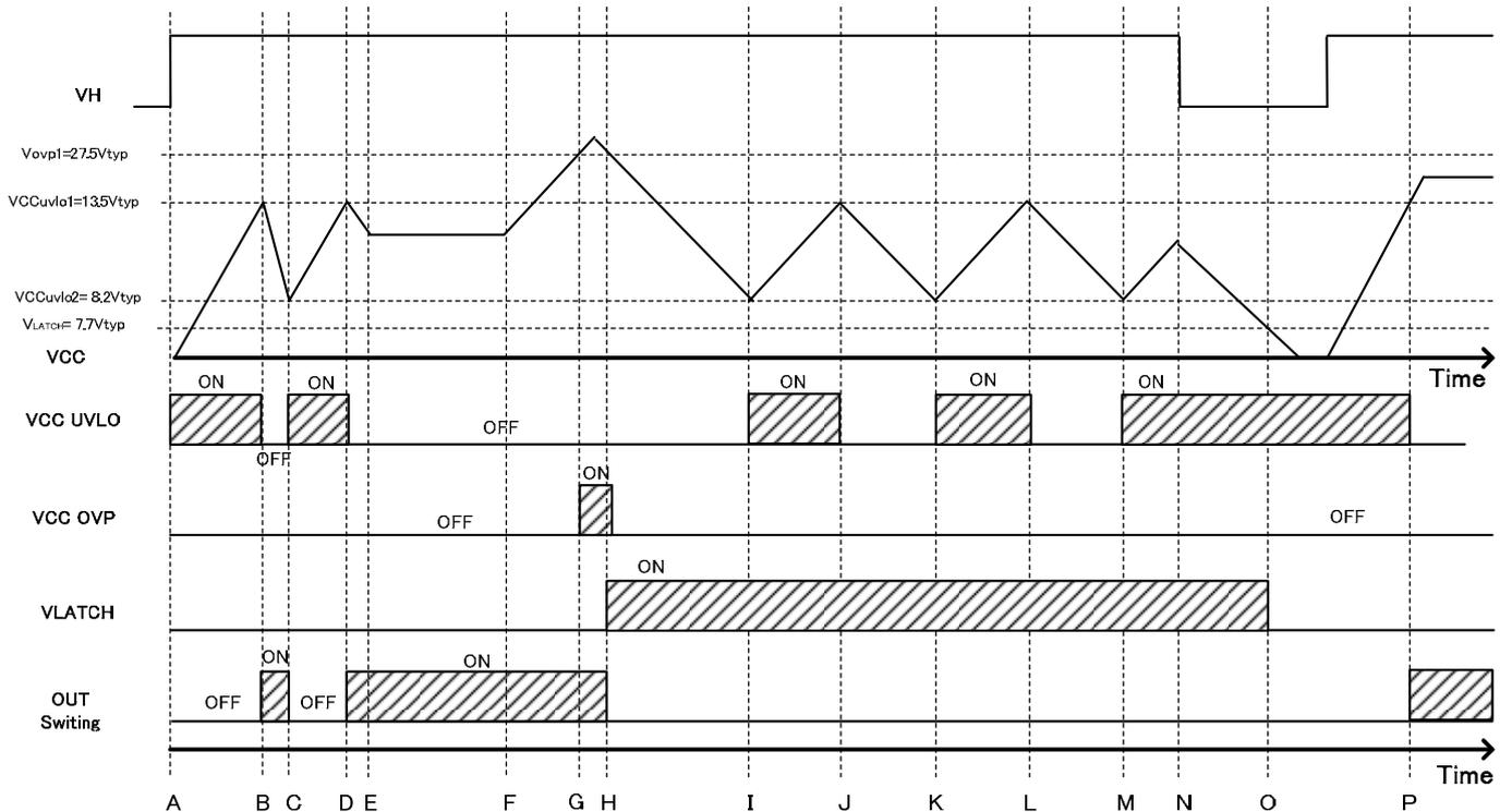
Figure 11. VCC UVLO / OVP Time Chart
