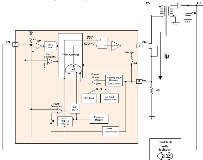
Figure 13. Block Diagram of IC Internal PWM Operations
