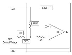
Figure 7. Sequencing Signal Interface of Module
