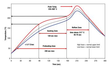
Recommended Lead-free Solder Reflow Profile
