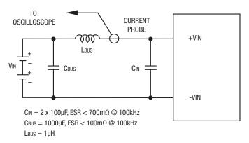
Figure 4. Measuring Input Ripple Current
