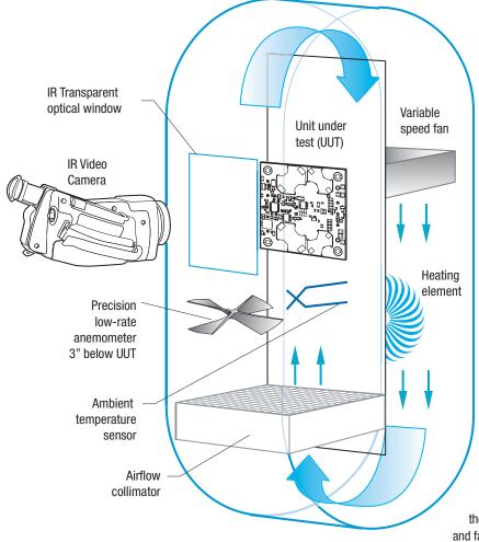
Figure 9. Vertical Wind Tunnel
