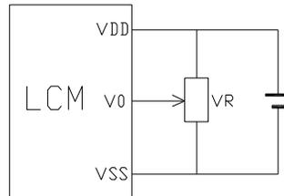
V<sub>DD</sub>-V<sub>0</sub>: LCD Driving voltage
