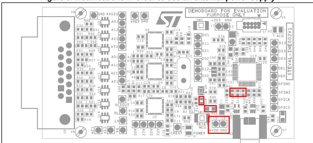
**Note:** Do NOT use 3.3 V pad (test point 17) to apply an external power supply.
