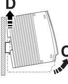
Figure 8 Removing the DIN rail
