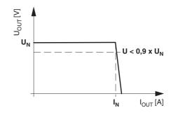
Figure 16 U/I characteristic curve
