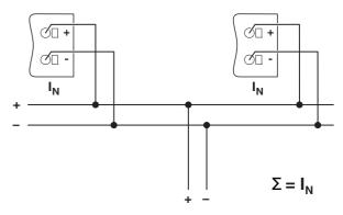
Figure 22 Schematic diagram in parallel operation
