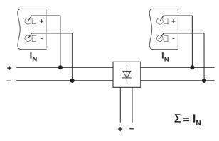
Figure 23 Schematic diagram, decoupling with diode module
