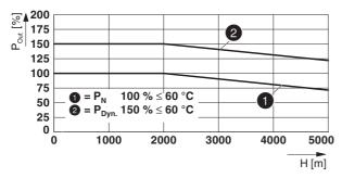
Figure 20 Output power depending on the installation height
