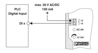
Figure 18 Wiring principle
