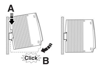
Figure 7 Assembly on standard DIN rail
