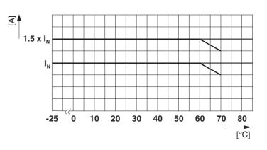
Rotated mounting position 90° X-axis
