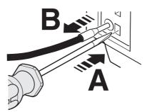
Figure 10 Release connecting cable (push-in connection technology)
