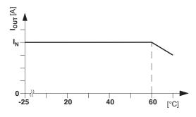
Figure 19 Temperature derating in normal mounting position
