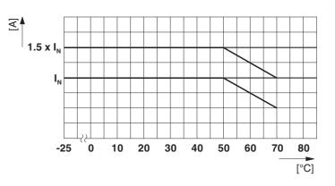
Rotated mounting position 270° X-axis
