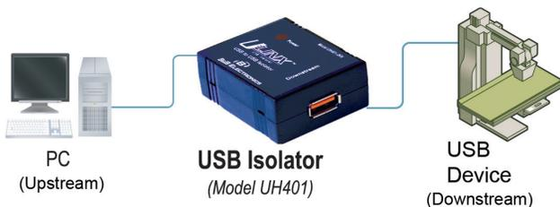
The USB isolator is transparent to the operating system. It will not appear in the device manager. Operation of the isolator can be verified by the “power ON” LED. This indicator illuminates when the device is plugged in to a 500 mA port.
