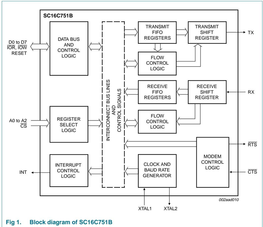
Fig 1. Block diagram of SC16C751B
