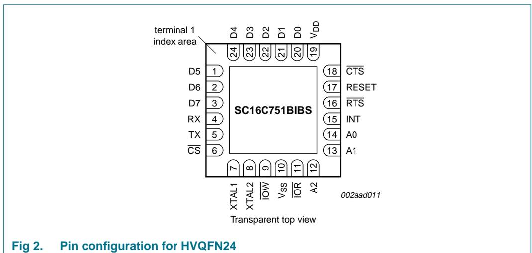
Fig 2. Pin configuration for HVQFN24
