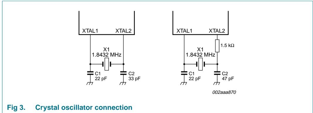
Fig 3. Crystal oscillator connection
