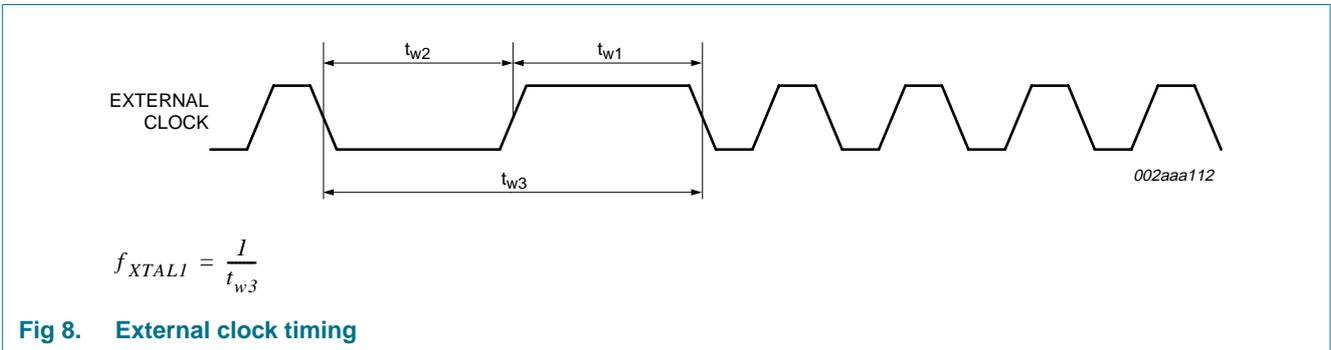
Fig 8. External clock timing
