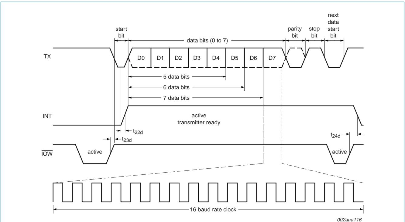
Fig 10. Transmit timing
