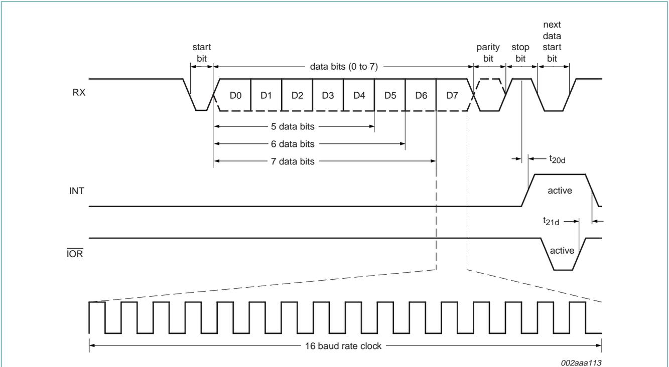
Fig 9. Receive timing
