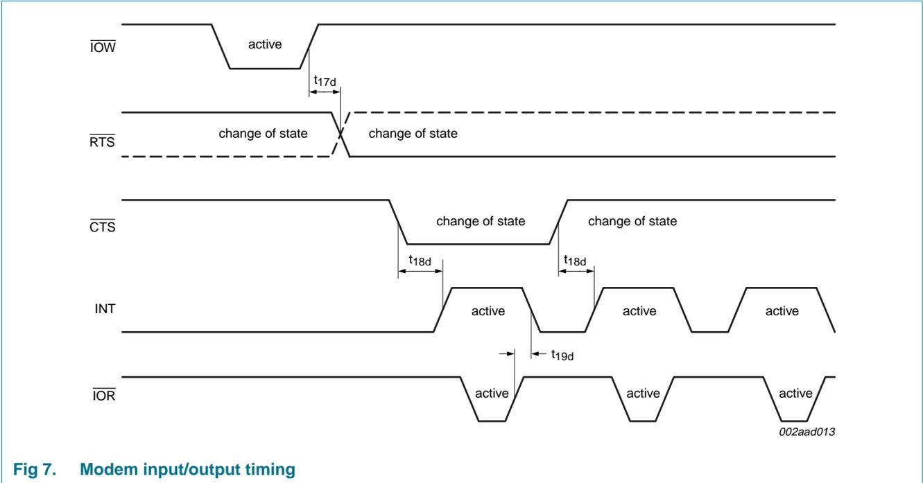
Fig 7. Modem input/output timing
