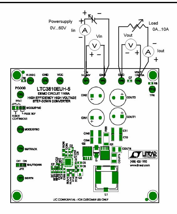
Figure 1. Proper Measurement Equipment Setup
