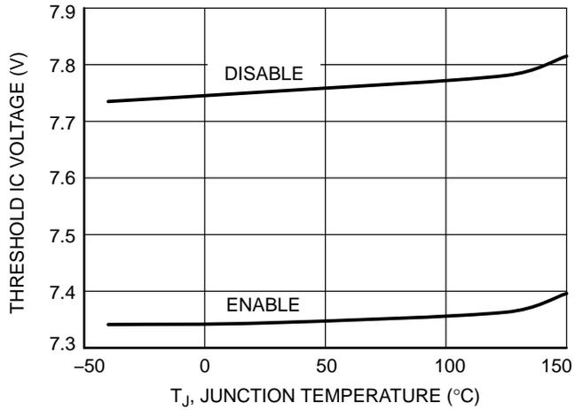
Figure 10. NCV887700/01 Threshold IC Voltage vs. Temperature
