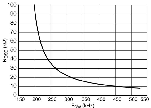
Figure 17. R<sub>osc</sub> vs. F<sub>sw</sub>
