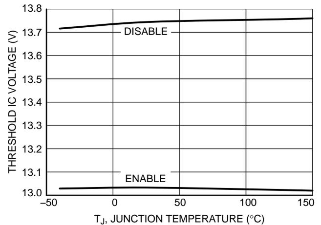
Figure 14. NCV887740 Threshold IC Voltage vs. Temperature
