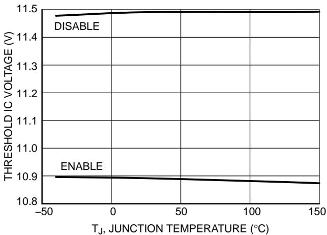
Figure 13. NCV887721 Threshold IC Voltage vs. Temperature
