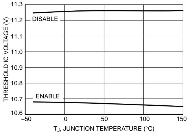
Figure 12. NCV887720 Threshold IC Voltage vs. Temperature
