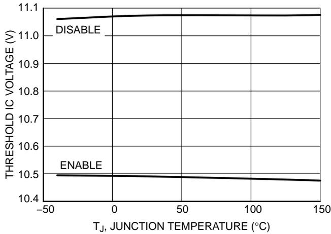
Figure 11. NCV887711 Threshold IC Voltage vs. Temperature
