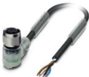
Sensor/actuator cable, 4-position, PUR halogen-free, black-gray RAL 7021, free cable end, on Socket angled M12 SPEEDCON, A-coded, with 3 LEDs, cable length: 1.5 m
