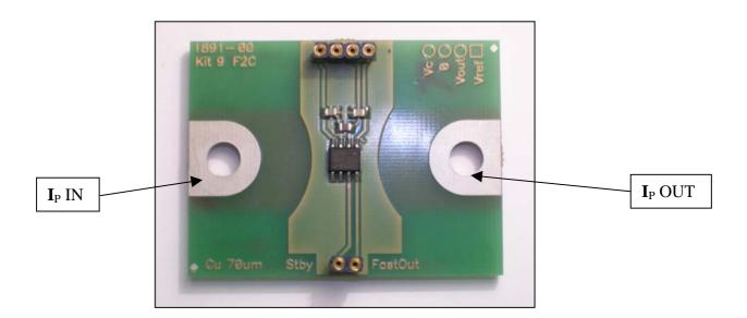
Connect then the primary between pins  $I_P$  IN and  $I_P$  OUT.
