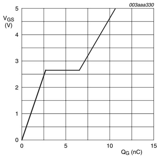
$I_D = 8A; V_{DD} = 15V$
