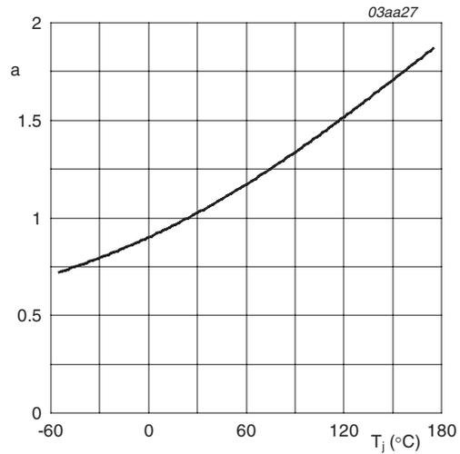
$$a = \frac{R_{DS(on)}}{R_{DS(on)(25^\circ C)}}$$
