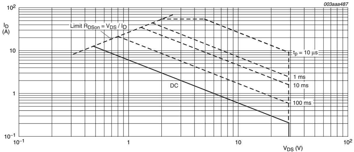
$T_{mb} = 25^\circ\text{C}; I_{DM}$  is single pulse
