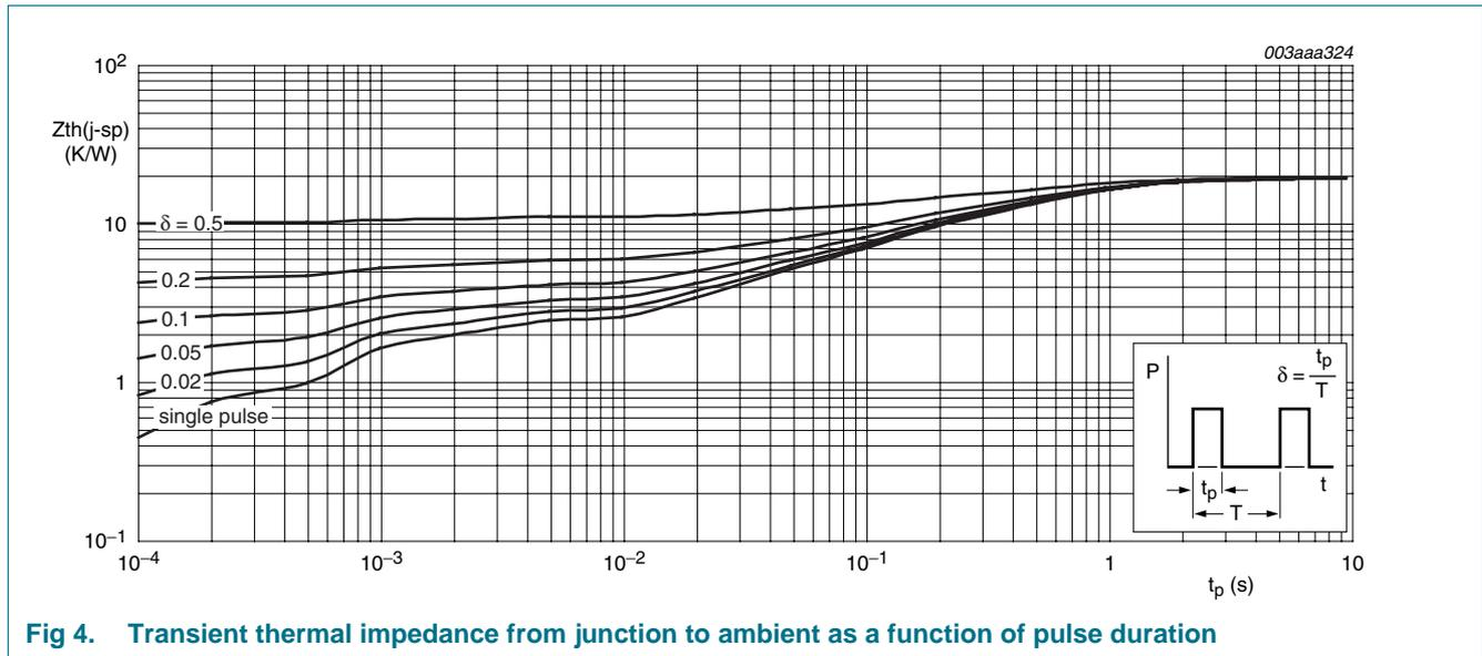
**Fig 4. Transient thermal impedance from junction to ambient as a function of pulse duration**
