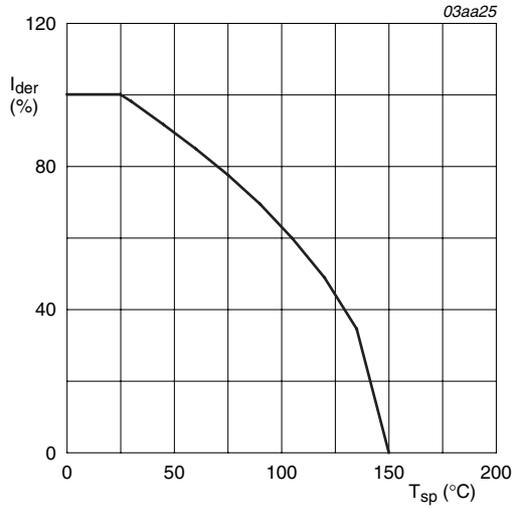
$$I_{der} = \frac{I_D}{I_{D(25^\circ\text{C})}} \times 100\%$$
