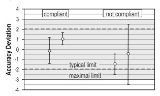
**Figure 3** Examples for accuracy distributions complying (left side) or not complying (right side) with the specified accuracy range. Open dots represent average values. Error bars denote 2k range and must stay within typical limits.
