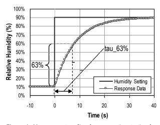
**Figure 4** Measurement profile of response time testing for relative humidity.
