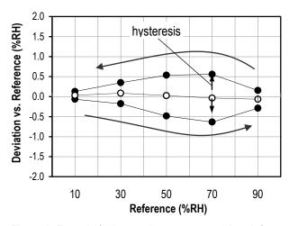
**Figure 2** Example for hysteresis measurement. A path from dry to humid and one from humid to dry is measured – full dots on graph. Dwell time at each log point is 30 minutes. Open dots determine mean values – representing calibration accuracy.
