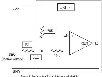
Figure 6. Sequencing Signal Interface of Module
