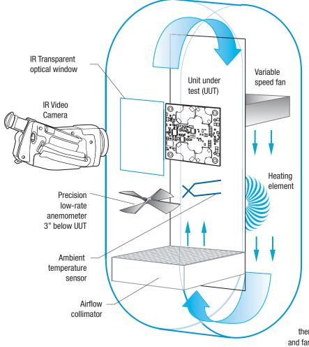
Figure 8. Vertical Wind Tunnel
