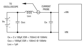
Figure 4. Measuring Input Ripple Current
