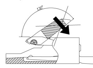
4. When operating the actuator, avoid operating it at its end. Make sure to operate it at its middle section.
