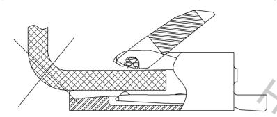
5. When inserting an FPC, do not use the method shown in the figure on the left below where the corner of the FPC is inserted first and then slid sideways. the FPC's corner can deform the terminal's contacts. Always insert the FPC parallel to the board as shown in the figure on the right below.
