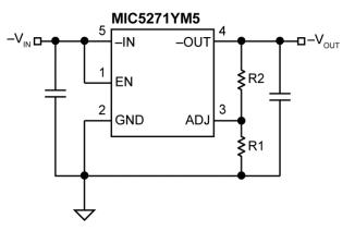
Figure 4. Adjustable Voltage Application
