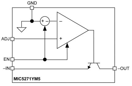
Figure 1. MIC5271YM5 (Adjustable Voltage)
