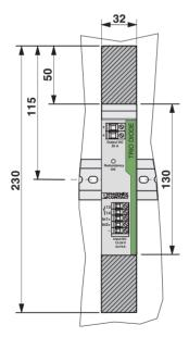
Mounting position: Installation depth 115 mm (+ DIN rail)
