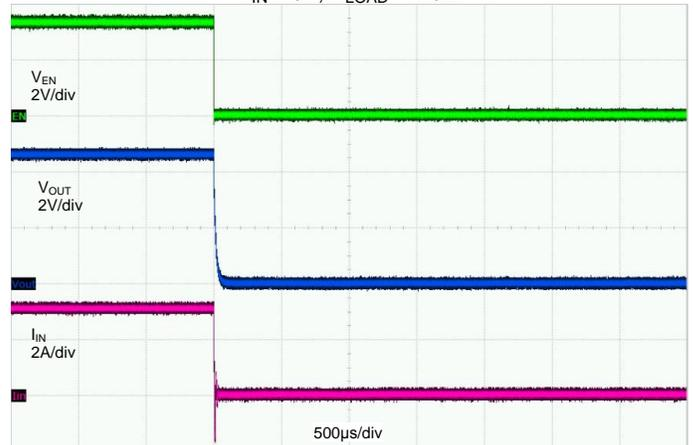
**EN Turn ON with a 7Ω Load at 20V**
