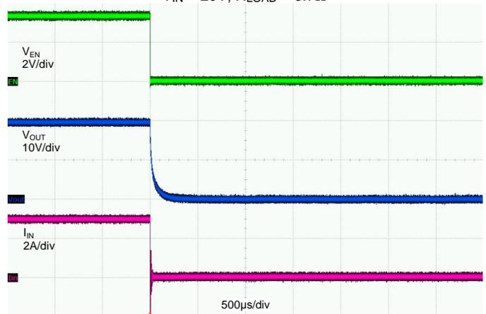
**Performance Characteristics** (continued) (@  $T_A = +25^\circ\text{C}$ ,  $C_{IN} = C_{OUT} = 10\mu\text{F}$ ,  $V_{EN} = 3.3\text{V}$ ,  $V_{FRS} = 0\text{V}$ ,  $C_{DV/DT} = 1\text{nF}$ ,  $R_{LIM} = 27\text{k}\Omega$ , unless otherwise specified)
