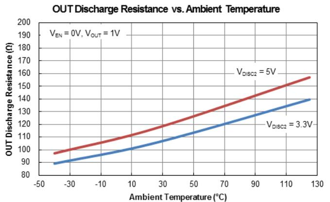
**Performance Characteristics** (continued) (@  $T_A = +25^\circ\text{C}$ ,  $C_{IN} = C_{OUT} = 10\mu\text{F}$ ,  $V_{EN} = 3.3\text{V}$ ,  $V_{FRS} = 0\text{V}$ ,  $C_{DV/DT} = 1\text{nF}$ ,  $R_{LIM} = 27\text{k}\Omega$ , unless otherwise specified)
