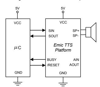
Basic Connection Diagram: Emic Platform with Microprocessor Host Control
