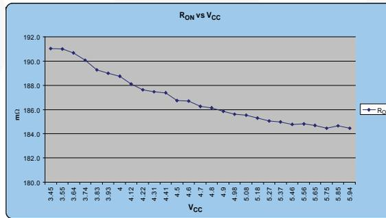
Figure 6. R<sub>ON</sub> vs. V<sub>CC</sub> (10Ω Load)
