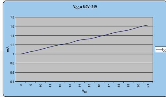
Figure 5. I<sub>CC</sub> vs. V<sub>CC</sub> (8.0V-21V) No Load
