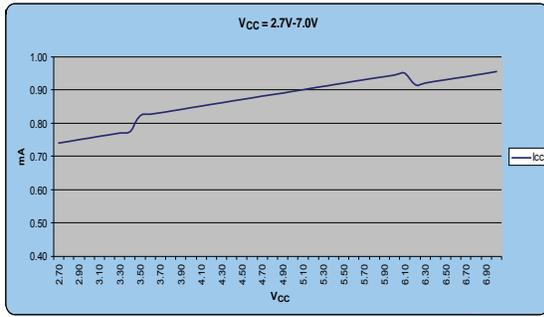
Figure 4. I<sub>CC</sub> vs. V<sub>CC</sub> (2.7V-7.0V) No Load
