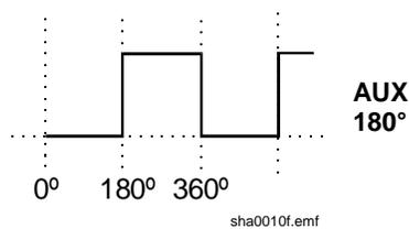
The convention adopted for phase in this instrument is illustrated in the diagram. 0° is always the first data point in waveform memory. On symmetrical waveforms 0° is the rising edge zero-crossing point for sine, square, triangle and pulse waveforms; on ramps, staircases and arbitrary waveforms 0° is always the start point.
