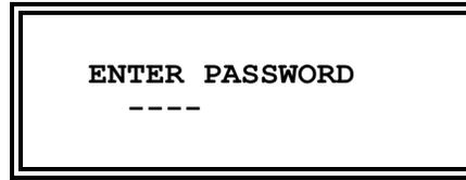
When the correct password has been entered from the keyboard the display changes to the opening screen of the calibration routine itself and calibration can proceed as described below under *Calibration Routine*. If an incorrect password is entered the message **INCORRECT PASSWORD!** is shown for two seconds before the display reverts to the main menu.
