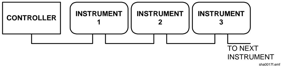
The daisy chain consists of the transmit data (TXD), receive date (RXD) and signal ground lines only. There are no control/handshake lines. This makes XON/XOFF protocol essential and allows the inter-connection between instruments to contain just 3 wires.
