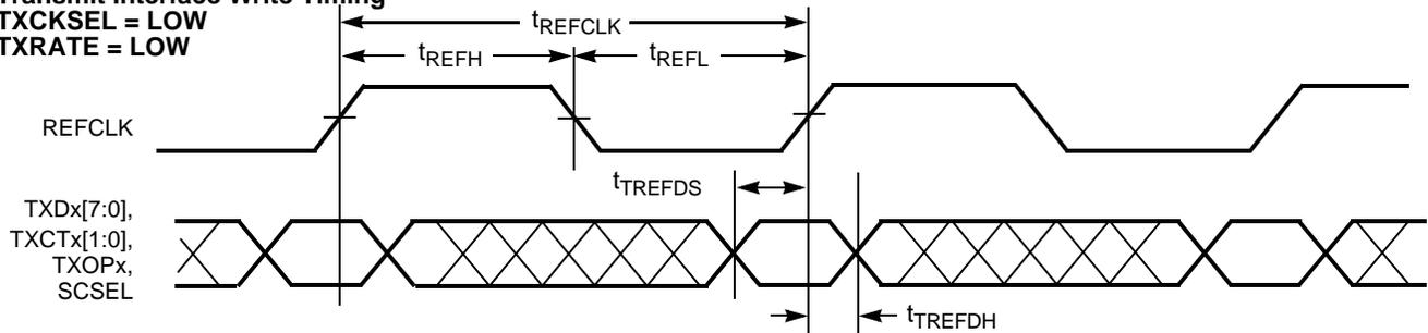
**Transmit Interface Write Timing
