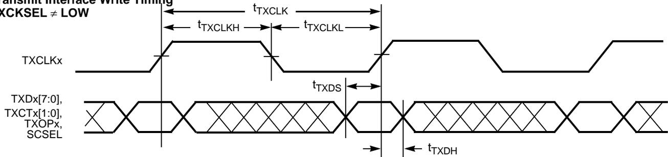
**Transmit Interface Write Timing
