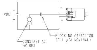
THE ABOVE RESULTS WILL ONLY BE ACHIEVED IF THE VDC SUPPLY HAS A VERY LOW INTERNAL IMPEDANCE AND IS CAPABLE OF ABSORBING RECYCLED ENERGY FROM THE RECEIVER.
