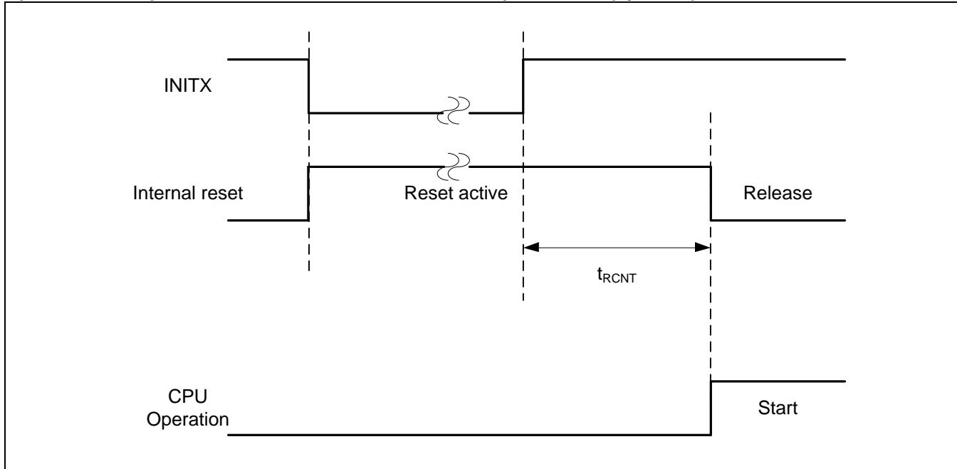
**Operation Example of Return from Low Power Consumption Mode (by Internal Resource Reset\*)**
