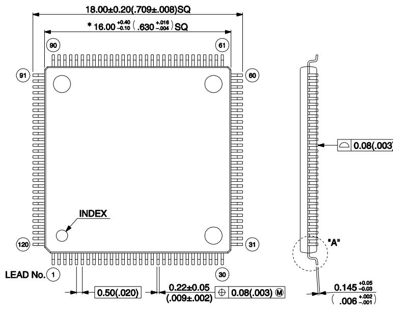
Note 1) \* : These dimensions do not include resin protrusion.
