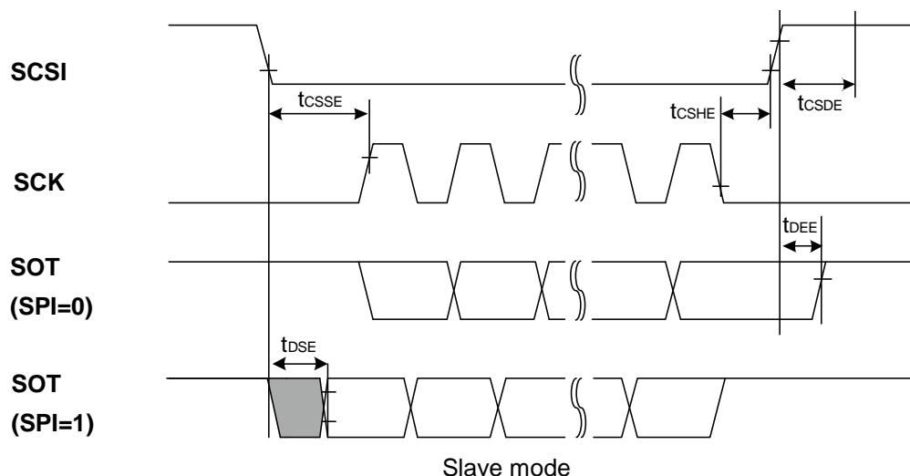
**When Using CSIO/SPI Chip Select (SCINV=0, CSLVL=0)**
