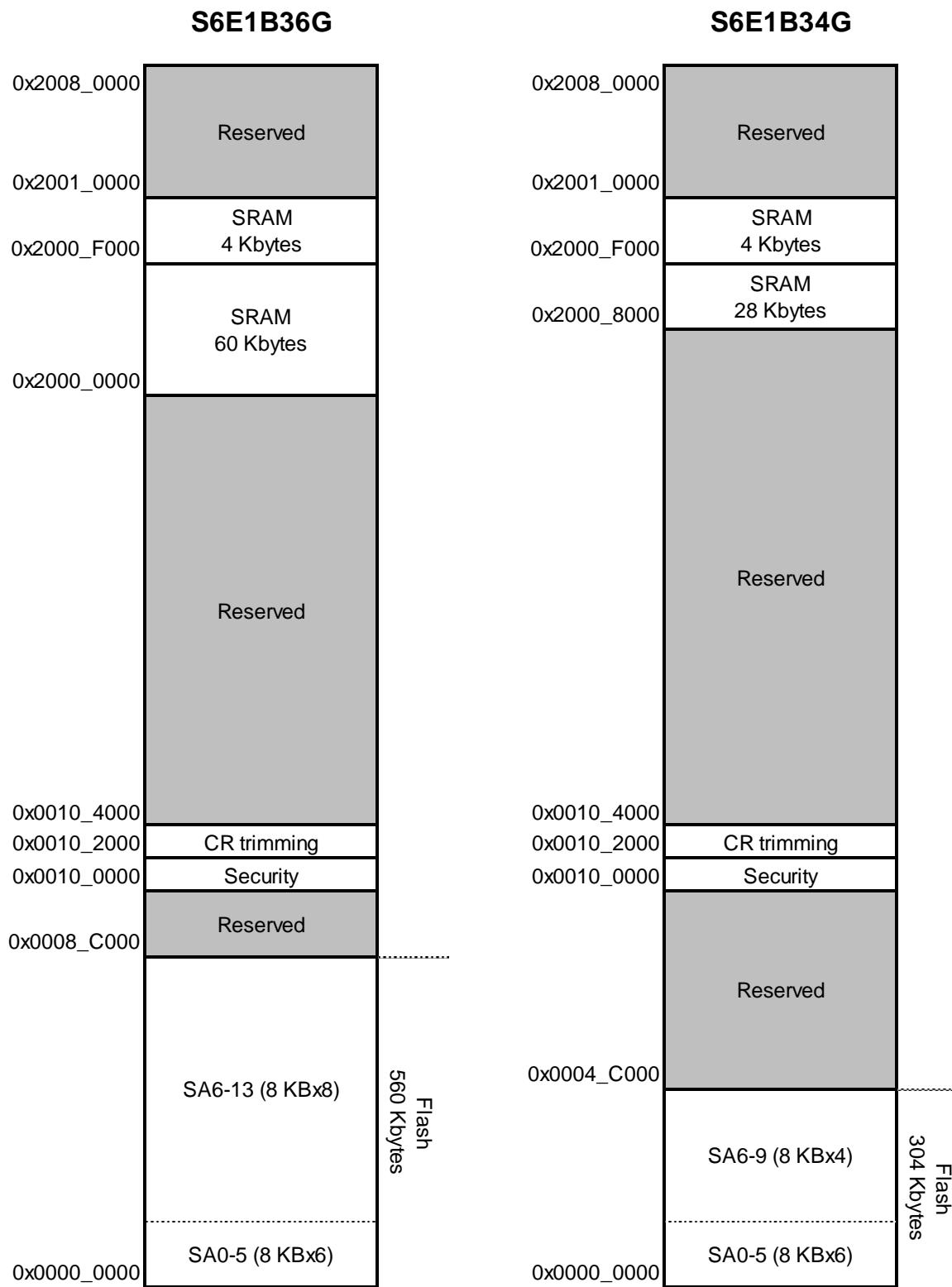
\*: See "S6E1B3 Series Flash Programming Manual" to check details of the Flash memory.
