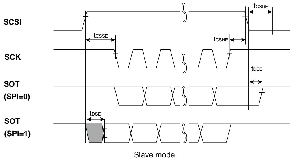
**When Using CSIO/SPI Chip Select (SCINV=1, CSLVL=0)**
