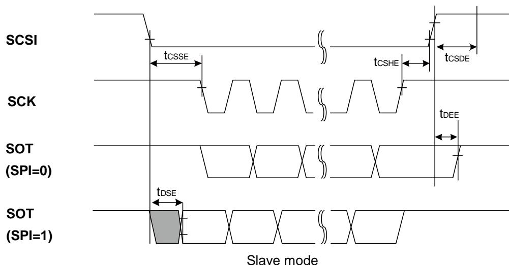
**When Using CSIO/SPI Chip Select (SCINV=1, CSLVL=1)**
