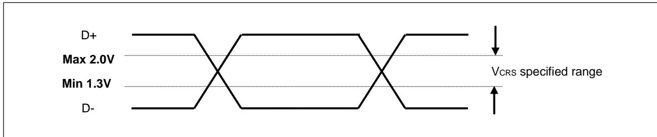
\*5 : The indicate rising time ( $T_{rise}$ ) and falling time ( $T_{fall}$ ) of the full-speed differential data signal.
