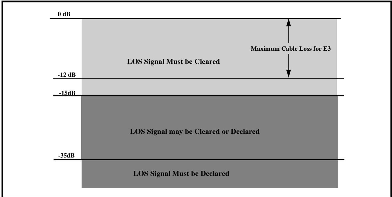
As defined in ITU-T G.775, an LOS condition is also declared between 10 and 255 UI (or E3 bit periods) after the actual time the LOS condition has occurred. The LOS condition is cleared within 10 to 255 UI after restoration of the incoming line signal. Figure 20 shows the LOS declaration and clearance conditions.
