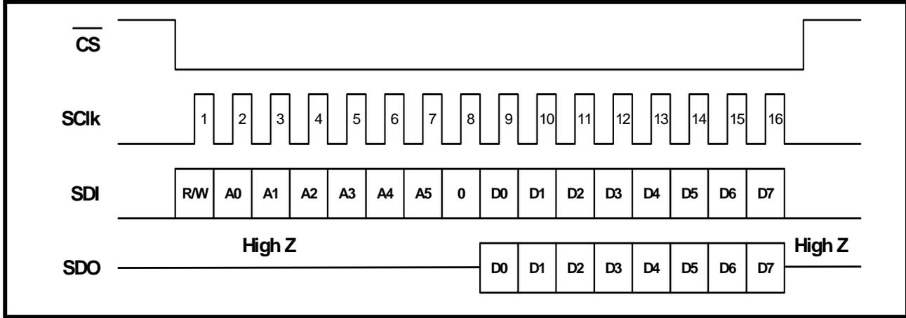
NOTE: If the R/W bit is set to "1", then this denotes a "READ" operation with the Microprocessor Serial Interface. Conversely, if the R/W bit is set to "0", then this denotes a "WRITE" operation.
