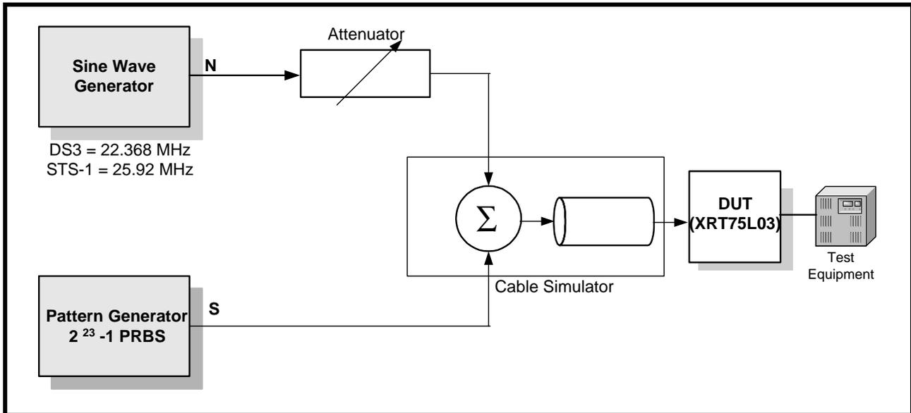
FIGURE 18. INTERFERENCE MARGIN TEST SET UP FOR E3.
