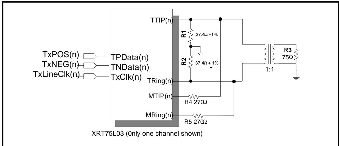
When the MTIP\_n and MRing\_n are connected to the TTIP\_n and TRing\_n lines, the drive monitor circuit monitors the line for transitions. The DMO\_n (Drive Monitor Output) will be asserted “Low” as long as the transitions on the line are detected via MTIP\_n and MRing\_n.
