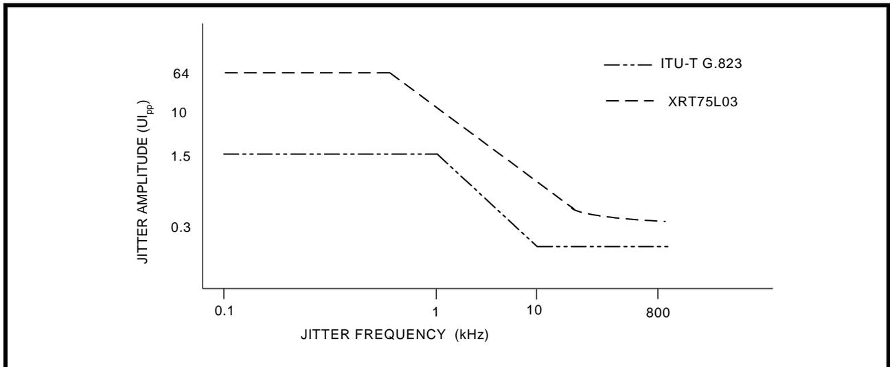
As shown in the Figures 22 and 23 above, in the jitter tolerance measurement, the dark line indicates the minimum level of jitter that the E3/DS3/STS-1 compliant component must tolerate.
