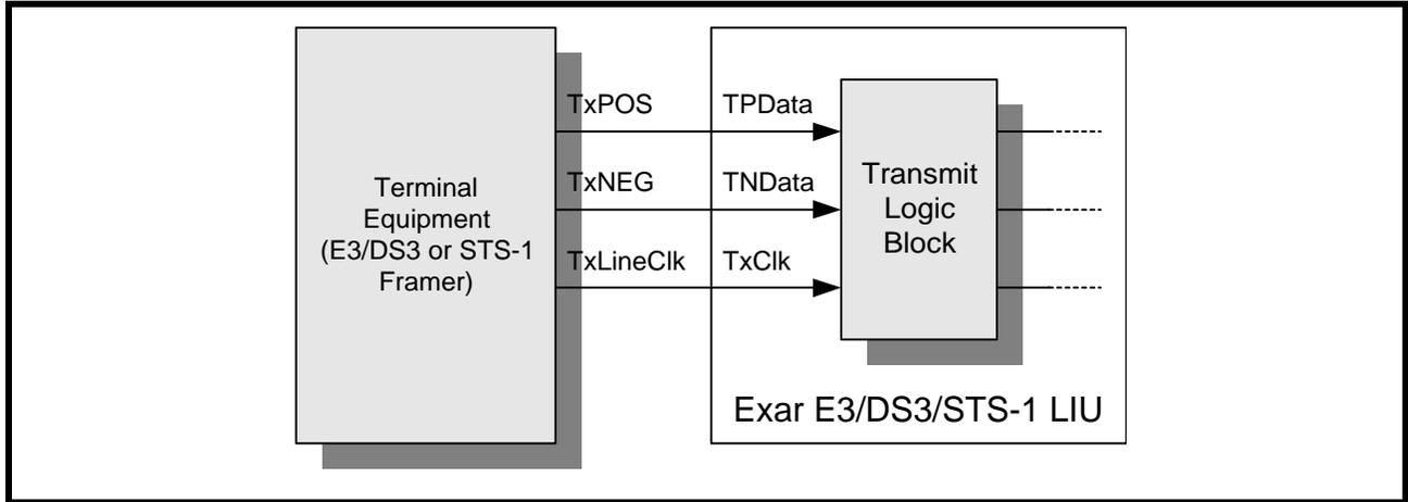
**FIGURE 4. TRANSMITTER TERMINAL INPUT TIMING**
