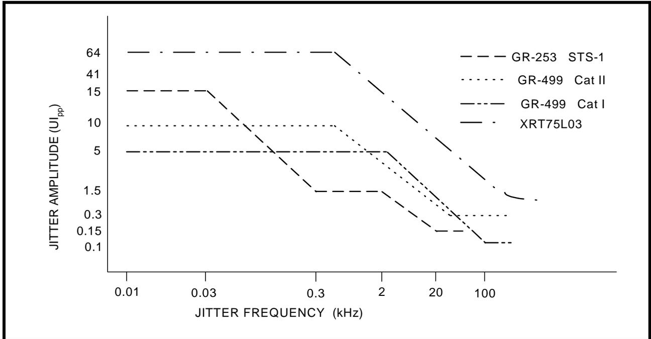
**6.1.2 E3 Jitter Tolerance Requirements:**
