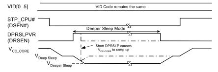
FIGURE 7. VCORE RESPONSE FOR DEEPER SLEEP COMMAND
