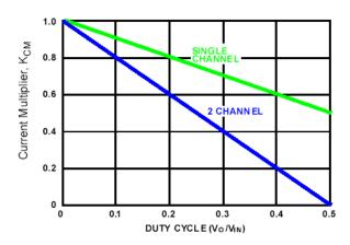
FIGURE 12. OUTPUT RIPPLE CURRENT MULTIPLIER vs DUTY CYCLE
