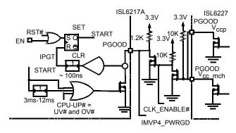
FIGURE 10. INTERNAL PGOOD CIRCUITRY FOR THE ISL6217A CORE VOLTAGE REGULATOR
