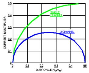
INPUT RMS CURRENT MULTIPLIER vs. DUTY
