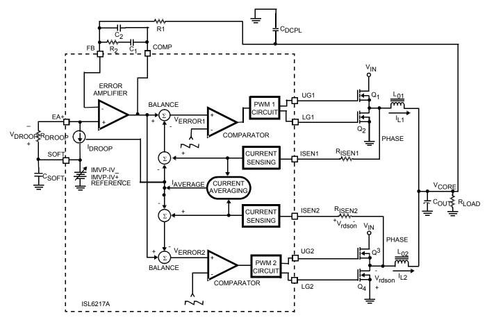
FIGURE 9. SIMPLIFIED BLOCK DIAGRAM OF THE ISL6217A VOLTAGE AND CURRENT CONTROL LOOPS FOR A TWO CHANNEL REGUL ATOR
