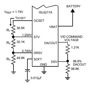
FIGURE 8. CONFIGURATIONS FOR BATTERY INPUT,
