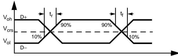
Figure 9-2. USB Data Signal Timing and Voltage Levels
