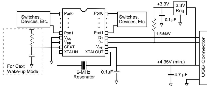
**Figure 6-28. Application Showing 1.5-k $\Omega$   $\pm$ 5% Pull-Up Resistor**
