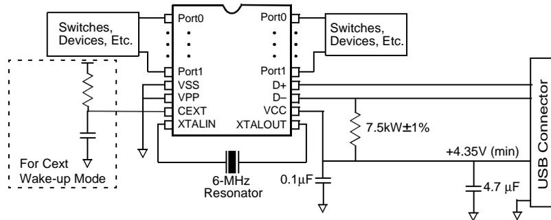
**Figure 6-27. Application Showing 7.5k $\Omega$   $\pm$ 1% Pull-Up Resistor**
