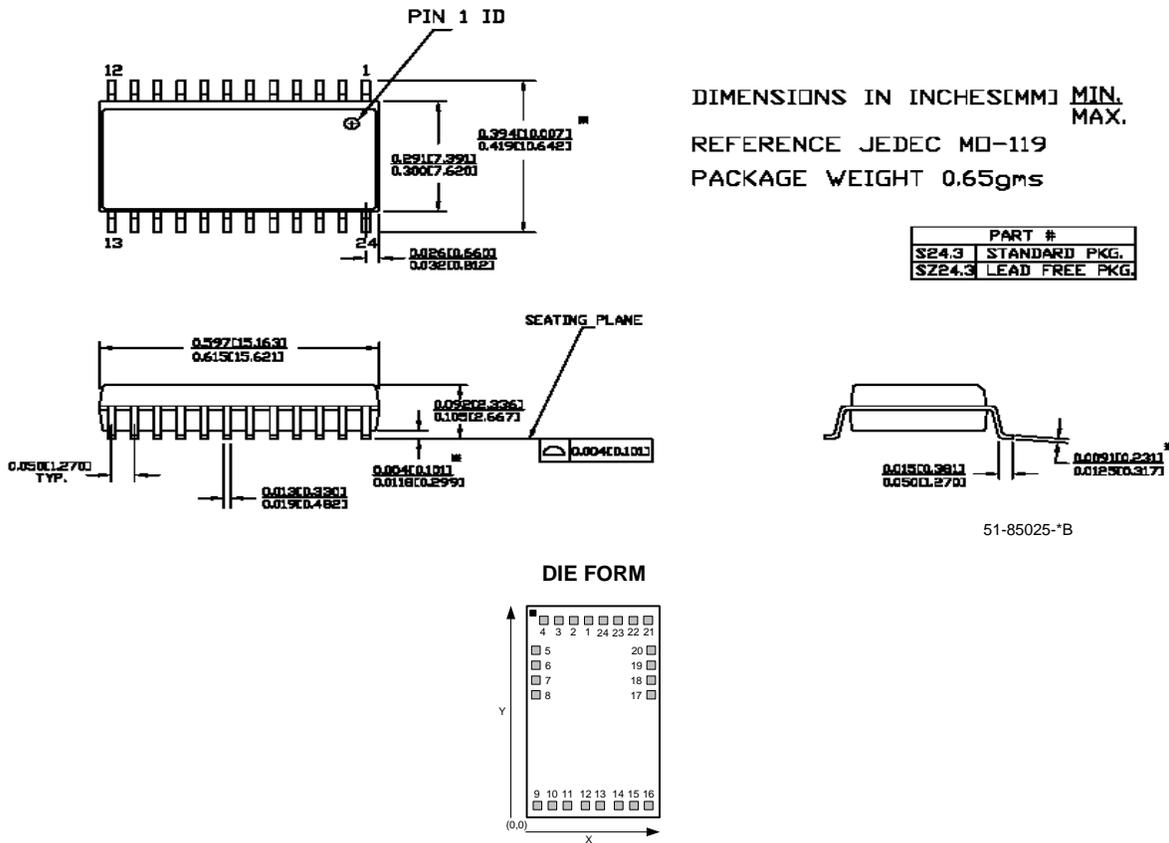
Table 11-1 below shows the die pad coordinates for the CY7C63001A-XC and CY7C63001A-XWC. The center location of each bond pad is relative to the bottom left corner of the die which has coordinate (0,0).
