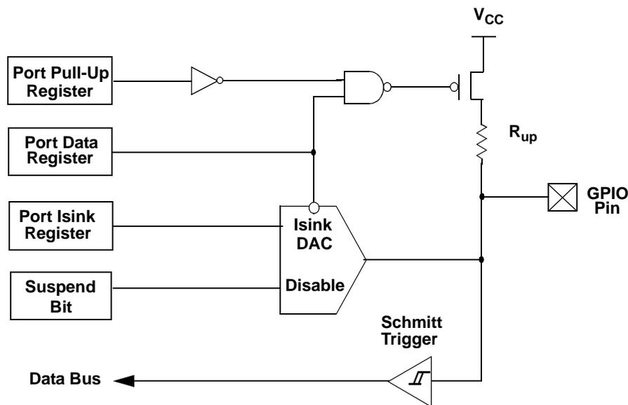
**Figure 6-10. Block Diagram of an I/O Line**
