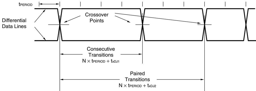
**USB differential-to-EOP transition skew and EOP width for low-/full-speed**
