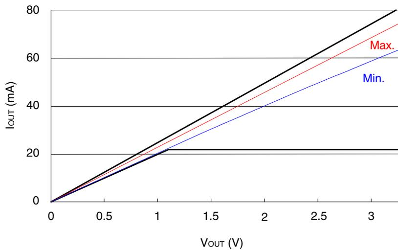
Figure 3-4. Receiver Sensitivity for Transceiver at DP/DM
