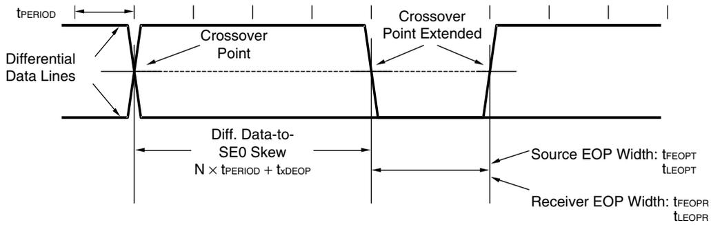
**USB receiver jitter tolerance for low-/full-speed**
