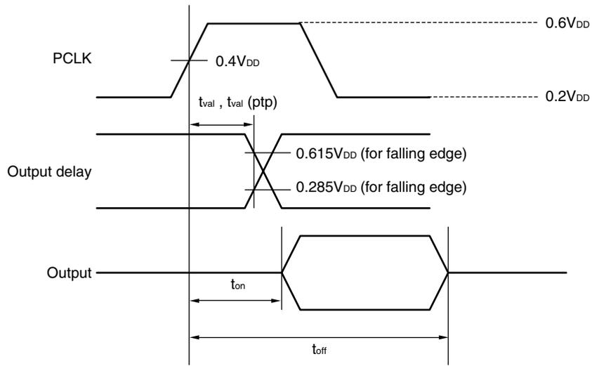
PCI input timing measurement condition
