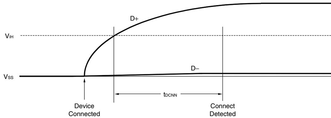
**Low-speed device connect detection**
