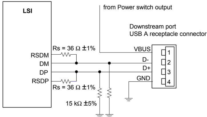
$R_s + R_{on}$  (Resistance for internal driver which is active) =  $45 \Omega \pm 10\%$
