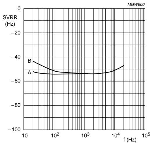
$V_{CC} = 12\text{ V}; R_{source} = 0\ \Omega; V_{ripple} = 707\text{ mV (RMS)}$ ; a bandpass filter of 10 Hz to 80 kHz has been applied.
