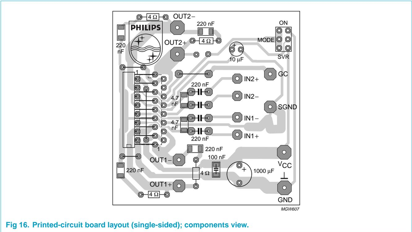
Fig 16. Printed-circuit board layout (single-sided); components view.
