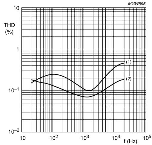
$V_{CC} = 12\text{ V}$ ; no bandpass filter applied
