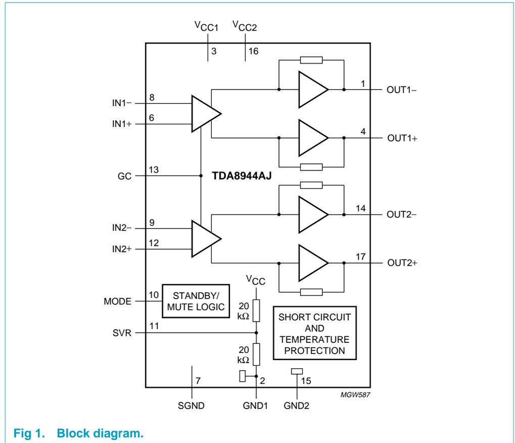
Fig 1. Block diagram.
