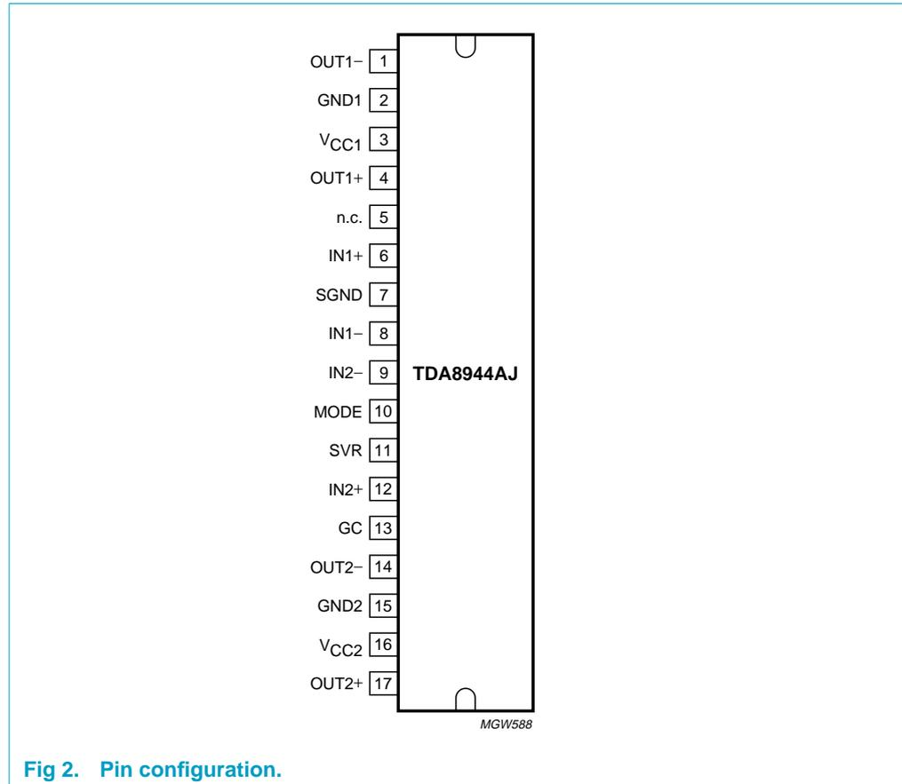
Fig 2. Pin configuration.
