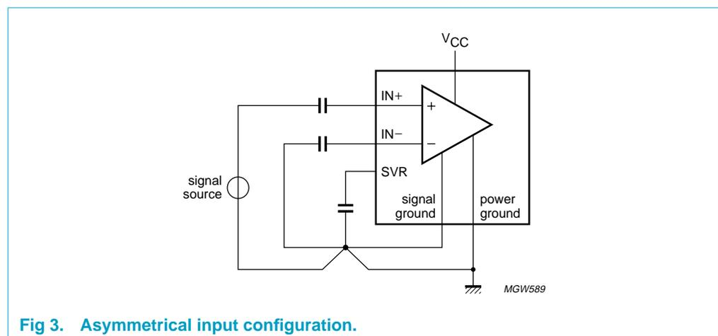
Fig 3. Asymmetrical input configuration.
